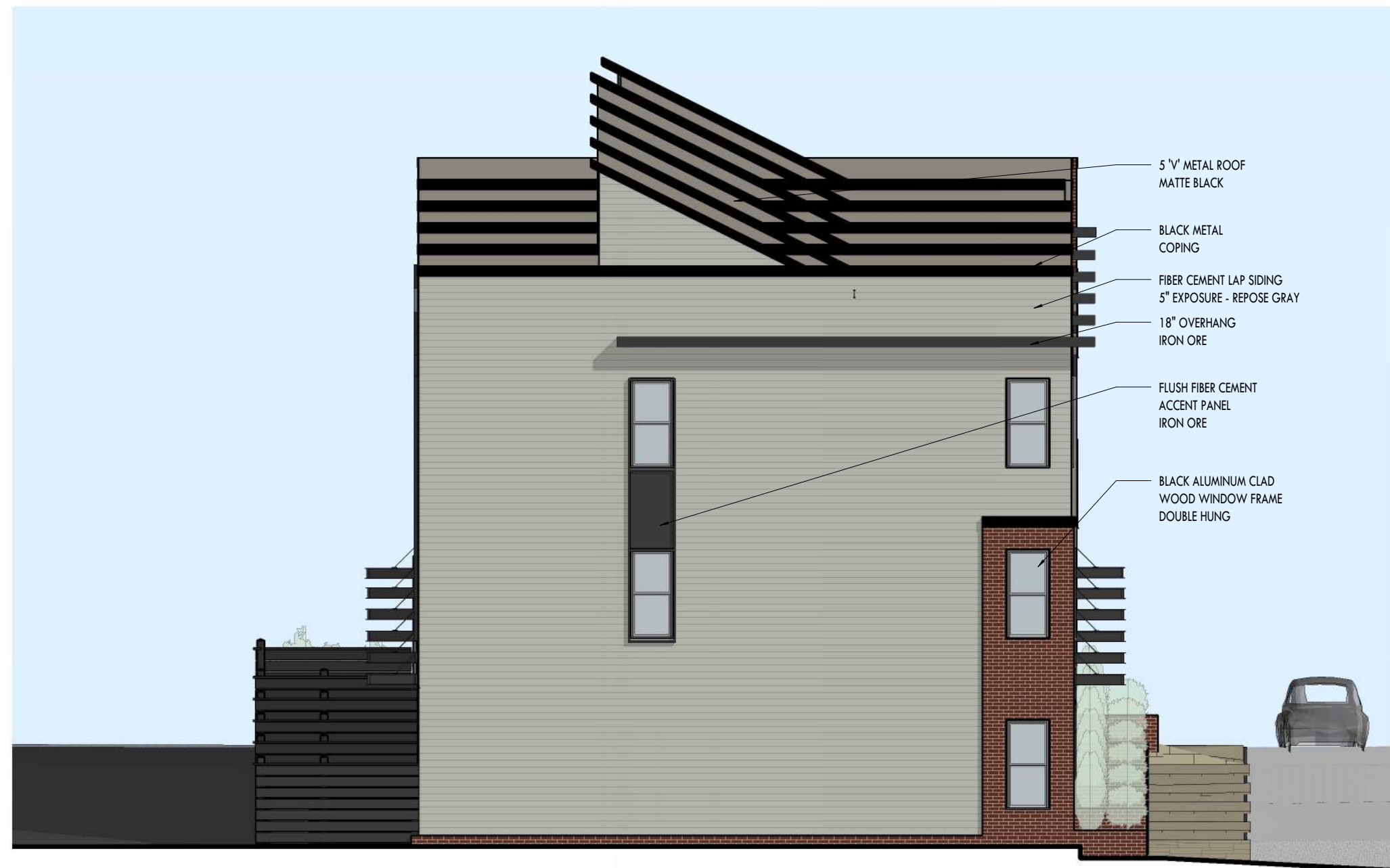
4 WEST ELEVATION 1/8" = 1'-0"
