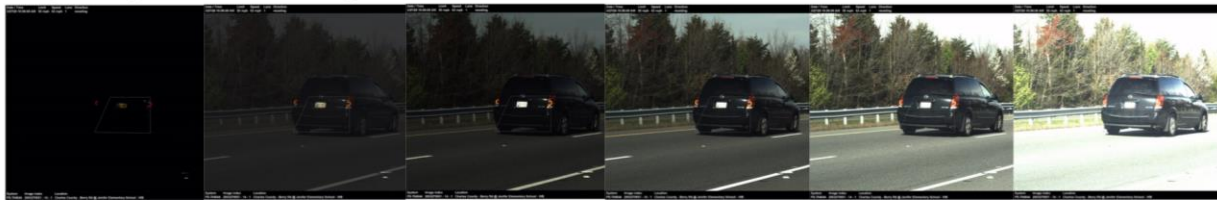
Figure 4.17.1-1 Image Exposure Example of high dynamic range of a single image
