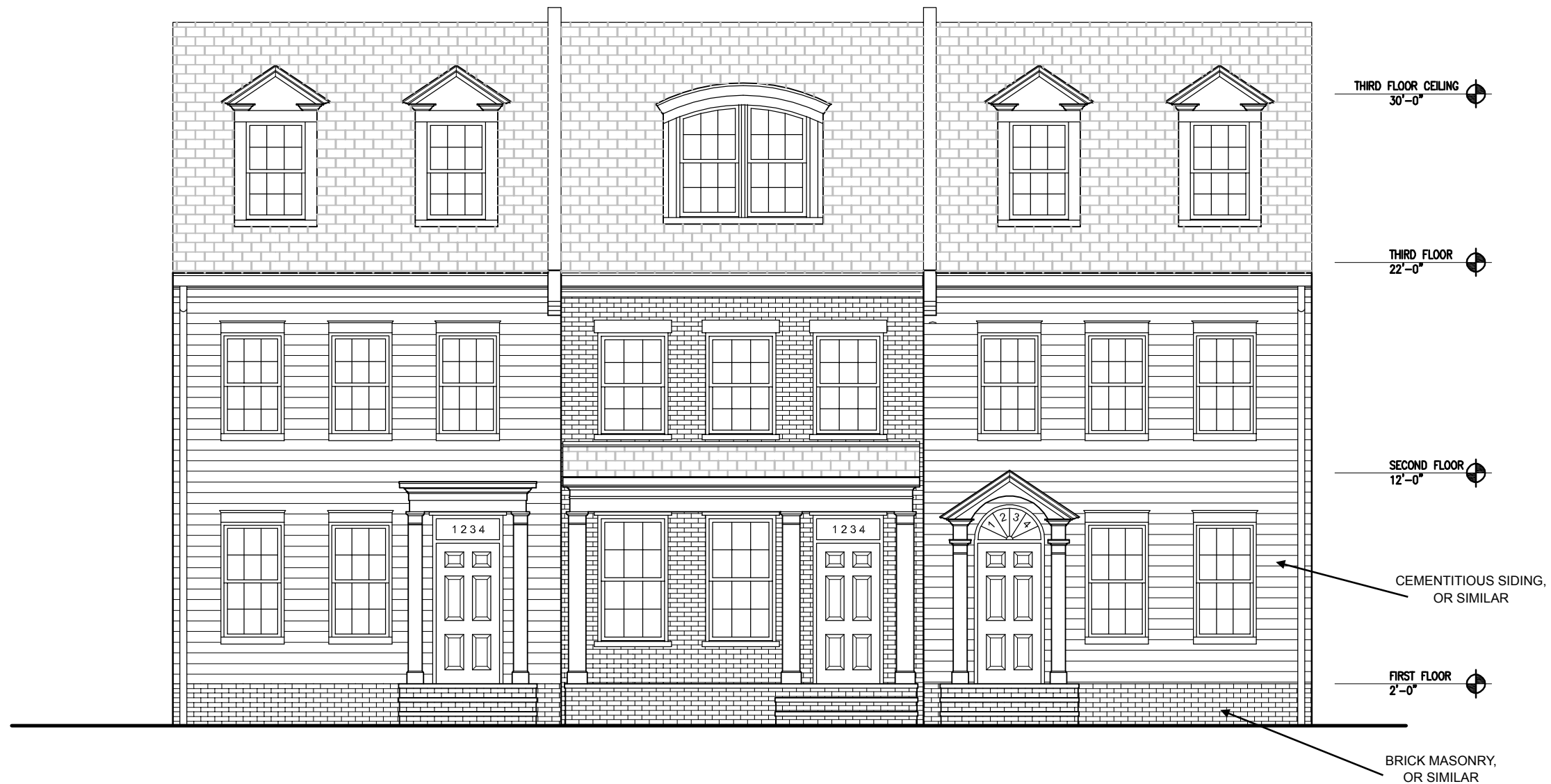
1 NORTH ELEVATION AT PATTERSON AVE SCALE: 1/4"=1'-0"
