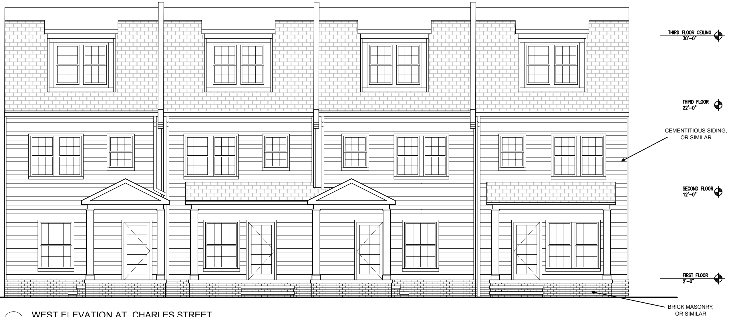
1 WEST ELEVATION AT CHARLES STREET SCALE: 1/4"=1'-0"
