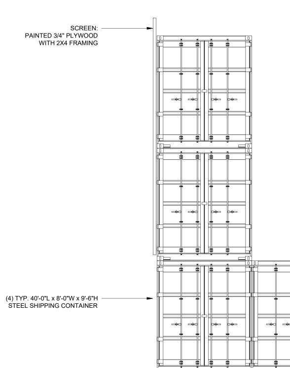
2 PROPOSED SCREEN ELEVATION - SIDE Scale: 1"= 1/4"
