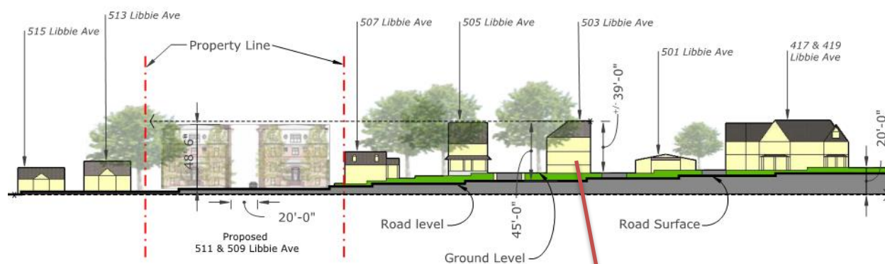
B 1 Libbie Avenue Longitudinal Section (looking east) This is a section in Sketchup using the contours layer from City GIS data and Pictometry to measure each existing building height
