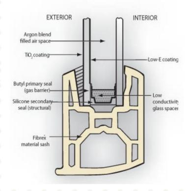
benefit of the air space diminishes and reduces the energy efficiency. If the two panes of glass are too far apart, convection can occur within the space, which provides a means of increasing heat loss instead of reducing it. Renewal by Andersen optimizes the space between the two glass panes for the best thermal performance.
