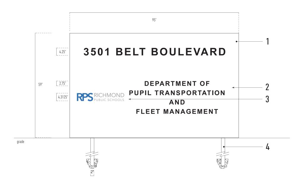
MOUNT: Buried no less than 24" below grade; filled with 3000 psi grade concrete
