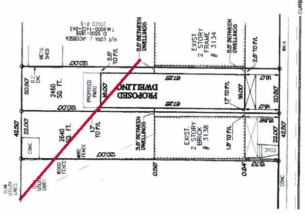
New proposed construction at 3136 would interrupt existing power lines at adjacent 3134 Grayland Ave, representing a disruption in service and a potential fire hazard as well as requiring service conducted on that adjacent property.
