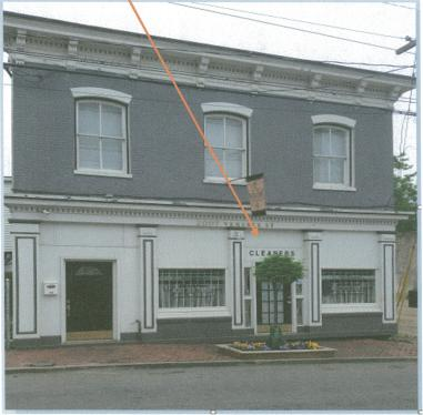
The illustrated canopy would go over the door pointed out. The dimensions of the canopy are Width 57", Projection 36", Height 35", and Height from sidewalk 7'6".
