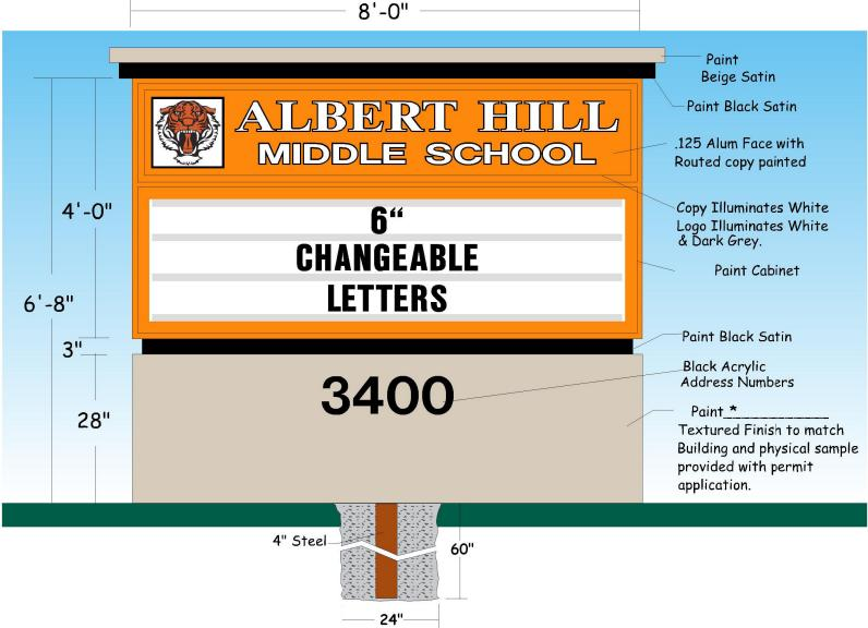
D/F Monument has 3 lines of 6" changeable copy with a clear lexan security door. Fabricated Aluminum Base\*painted Akzo Nobel 504-C1 Textured Finish to match Building.
