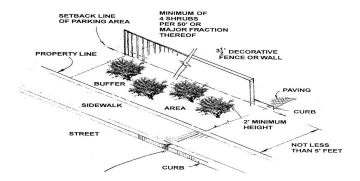
[9. Buffer "I," as shown below, shall have a depth of not less than two feet and shall include a decorative fence or wall not less than 3½ feet in height and vegetative ground cover, shrubs or other plant material.]
