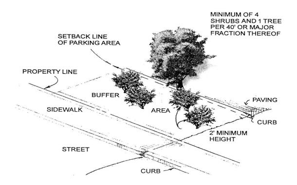
Buffer area depth dependent on yard requirement in district, but in no case less than five feet. Where yard requirement is five feet or less, trees and shrubs may be substituted as specified for [buffers "H," "I," or "J,"] buffer "H."
