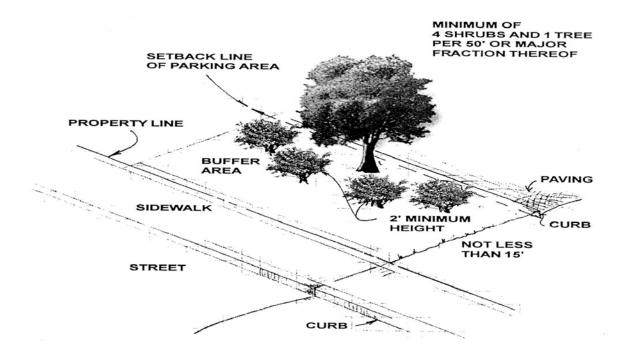
7. Buffer "G," as shown below, shall have a depth of not less than ten feet and shall include trees and shrubs at a rate of not less than one tree and four shrubs for each 40 linear feet or major fraction thereof of buffer along each street frontage.
