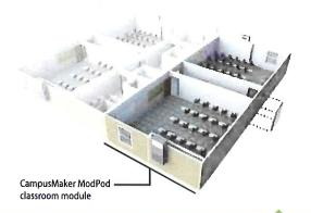
To adjust the size of the CampusMaker ModPod, the two classroom module at either end can be detached and relocated to another site or school, Construction of a new exterior wall is not required as the wall and finishes are already in place. This feature minimizes the down time due to construction and disjunction to the remainder of the classroom complex.
