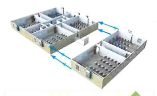
By simply removing and relocating the existing security entrance doors to the newly expanded CampusMaker ModPod, this classroom complex is set to operate with six classrooms, a restroom module and corridor. All this can be accomplished with minimal disruption to the occupants and in most cases, the work can be completed in just a few days.
