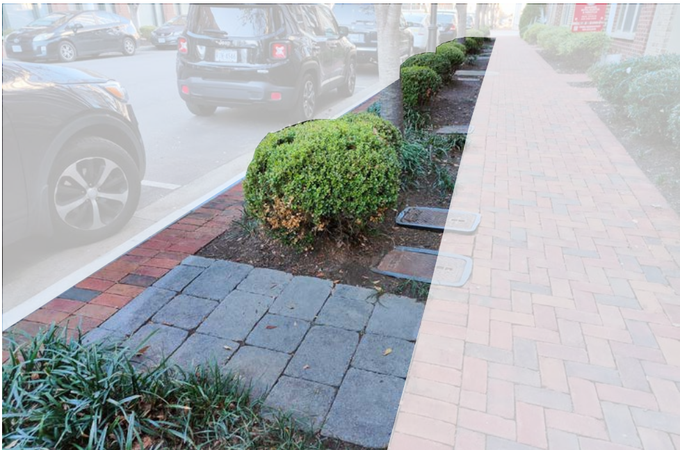
Tree wells are set back from the curb to allow for unobstructed access from the car, with periodic paver sections for pedestrian access.
