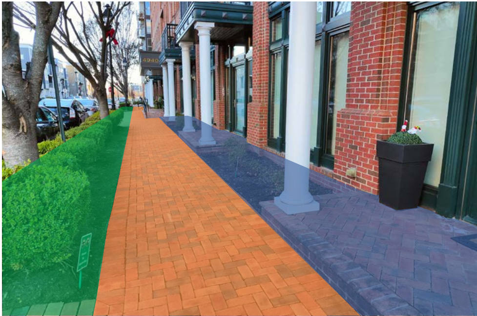
Design elements, such as columns, elevation change and landscaping create a clear delineation between each sidewalk zone.
