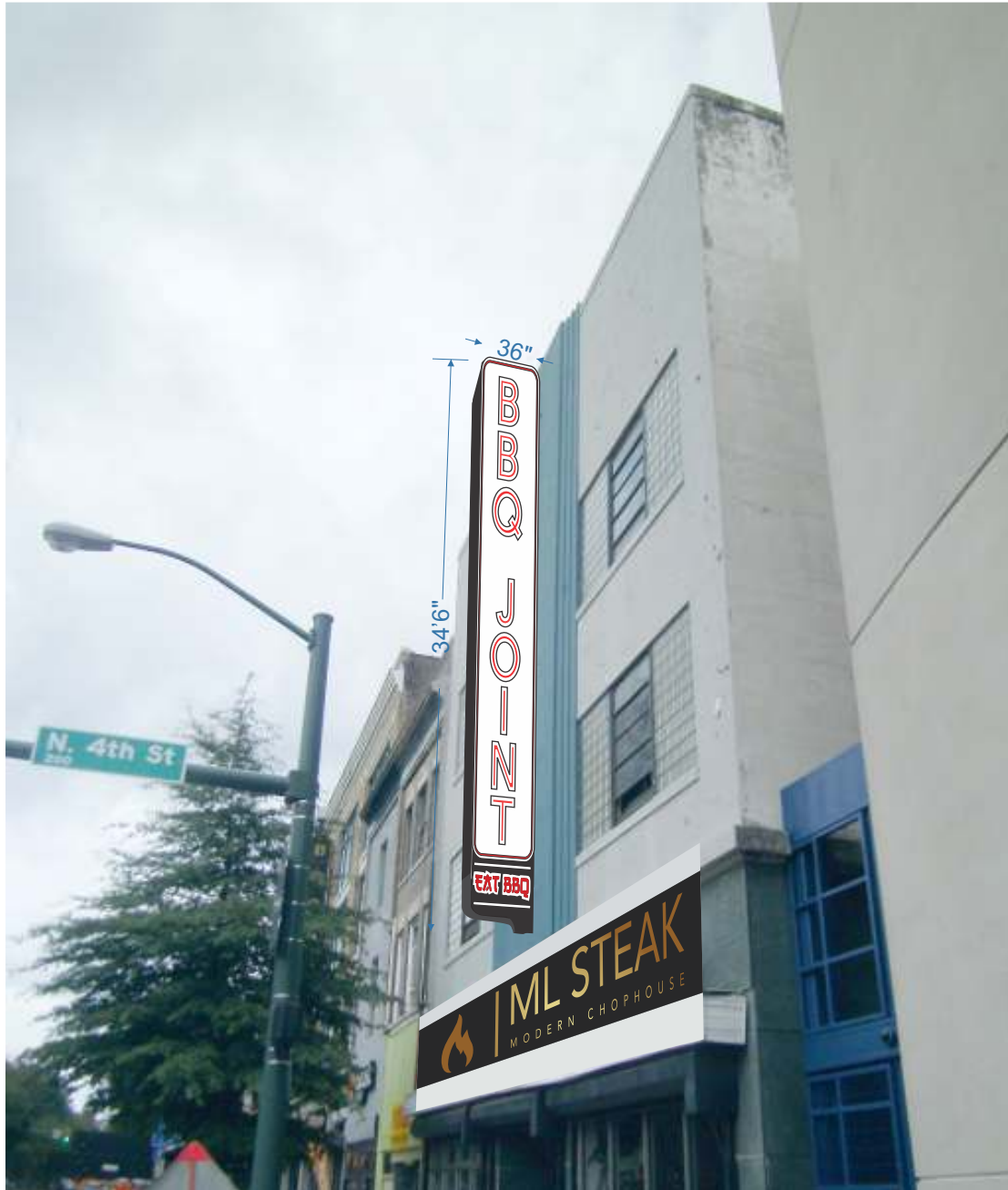
Channel letters neon sign. Channel letters with neon lights, black trim cap with clear faces, black returns. Sizes and colors as depicted on the drawing.
