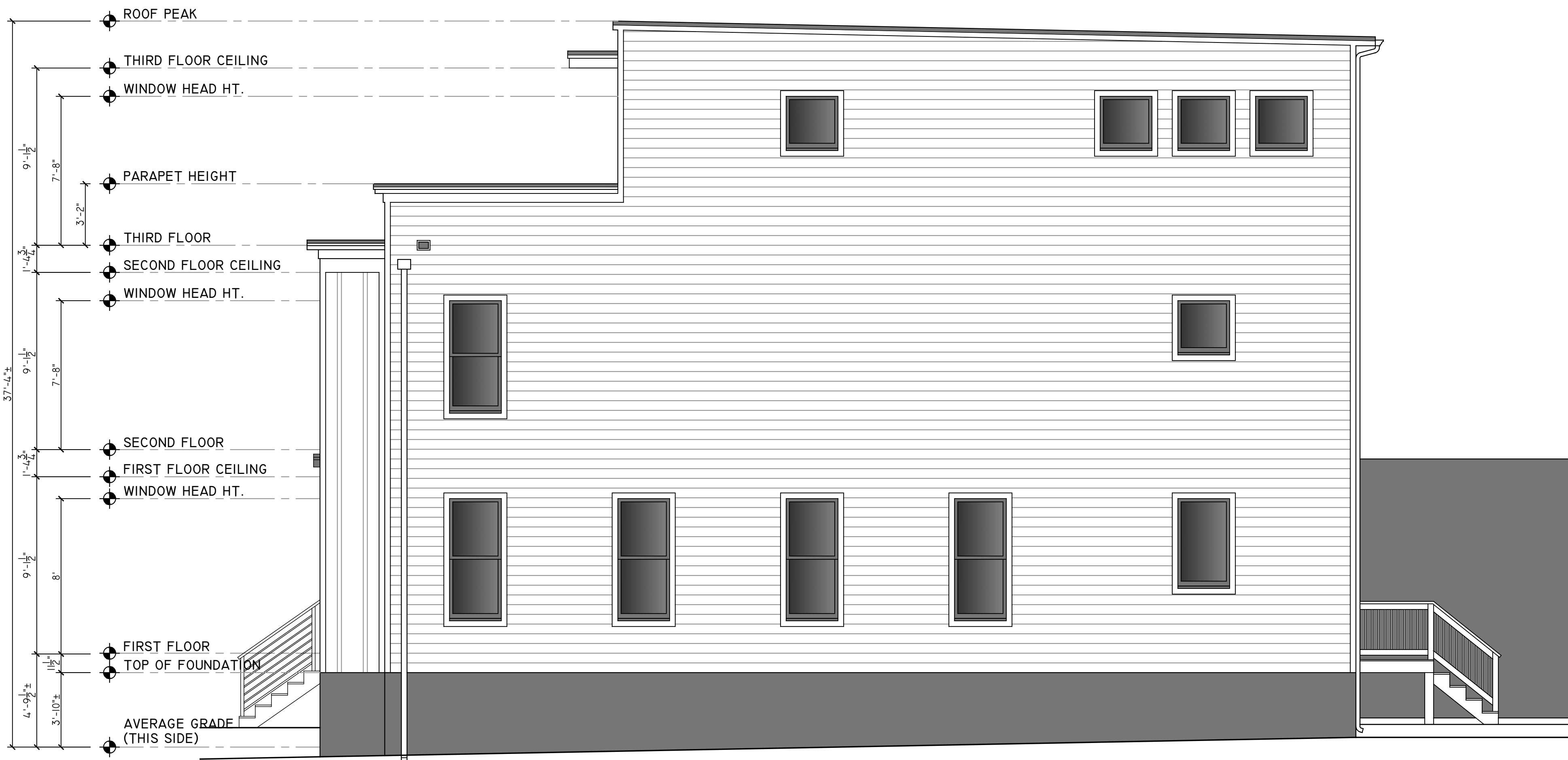
01 | RIGHT SIDE ELEVATION 1/4" = 1'
