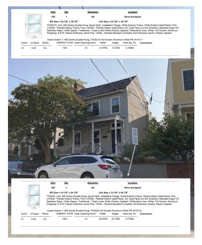
Addition of two accessory windows on the north elevation, flanking the chimney. Andersen, wood, fixed, no divided lights. Same trim style/width as existing.
