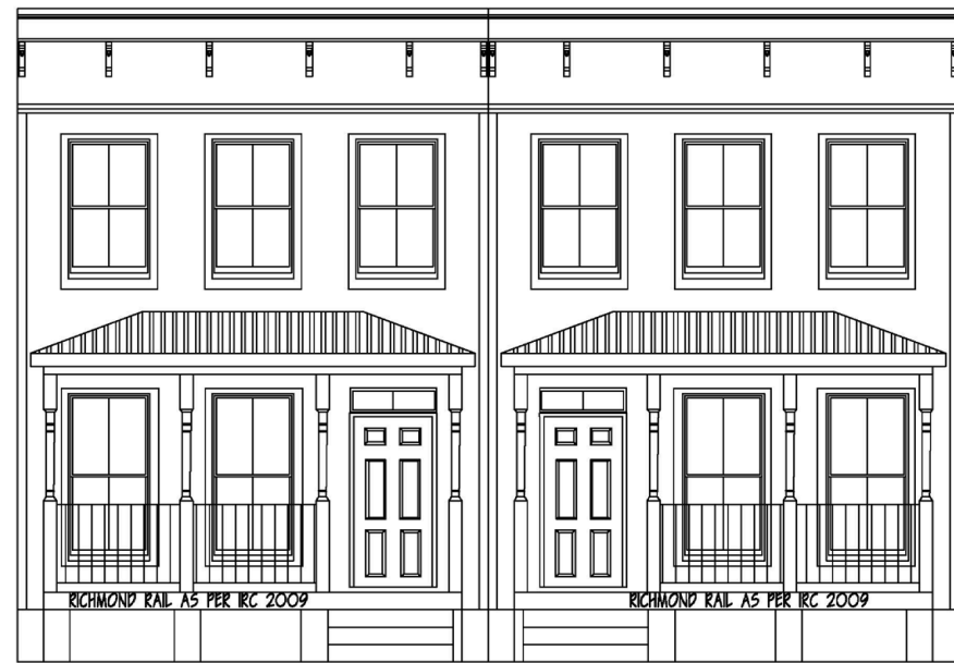
FOUNDATION HEIGHT NEEDS TO BE EQUAL OR LOWER THAN NEIGHBOR TO RIGHT Front Elevation Scale 1/4"=1'
