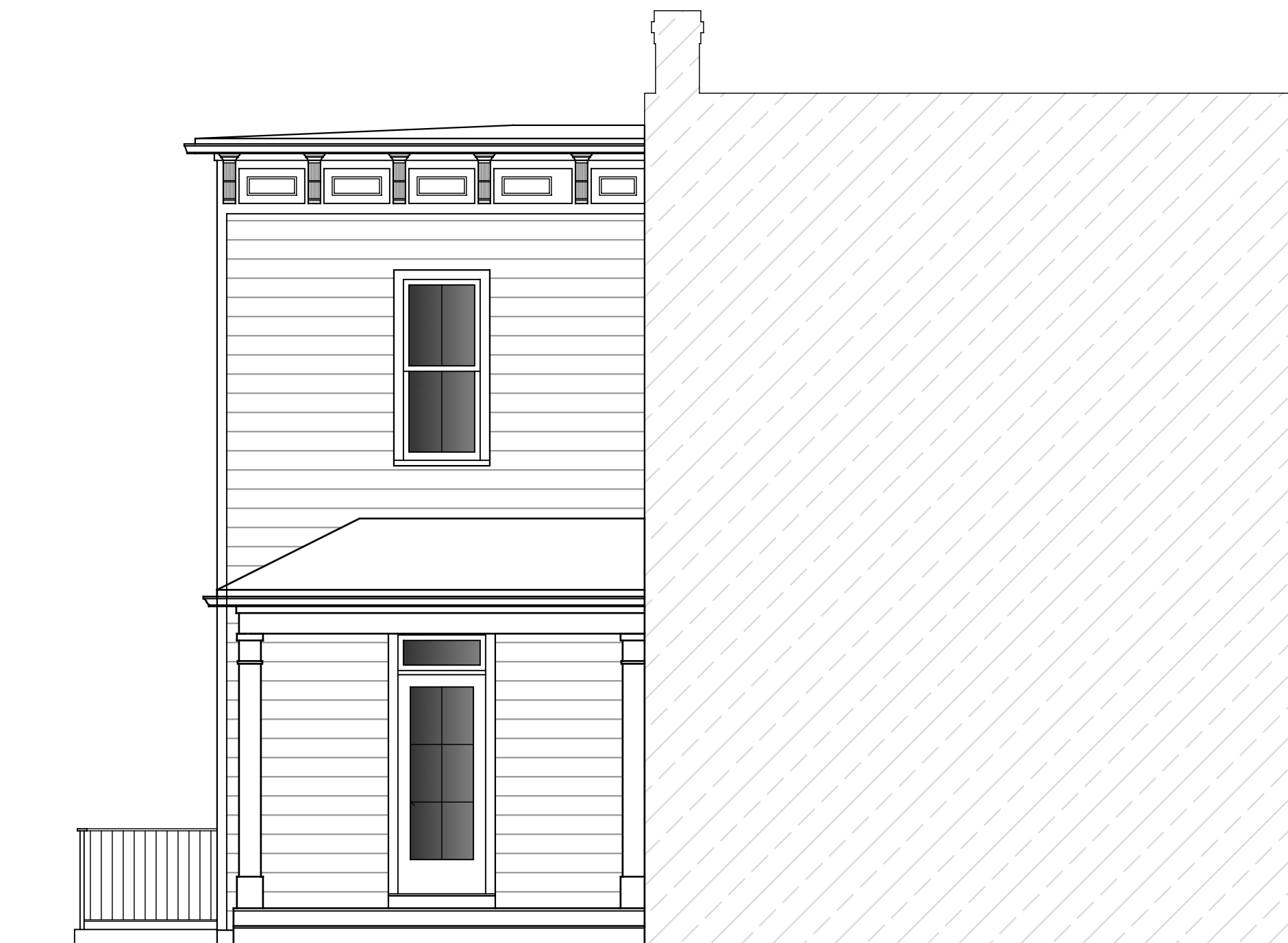
01 | NEW FRONT PORCH ELEVATION
