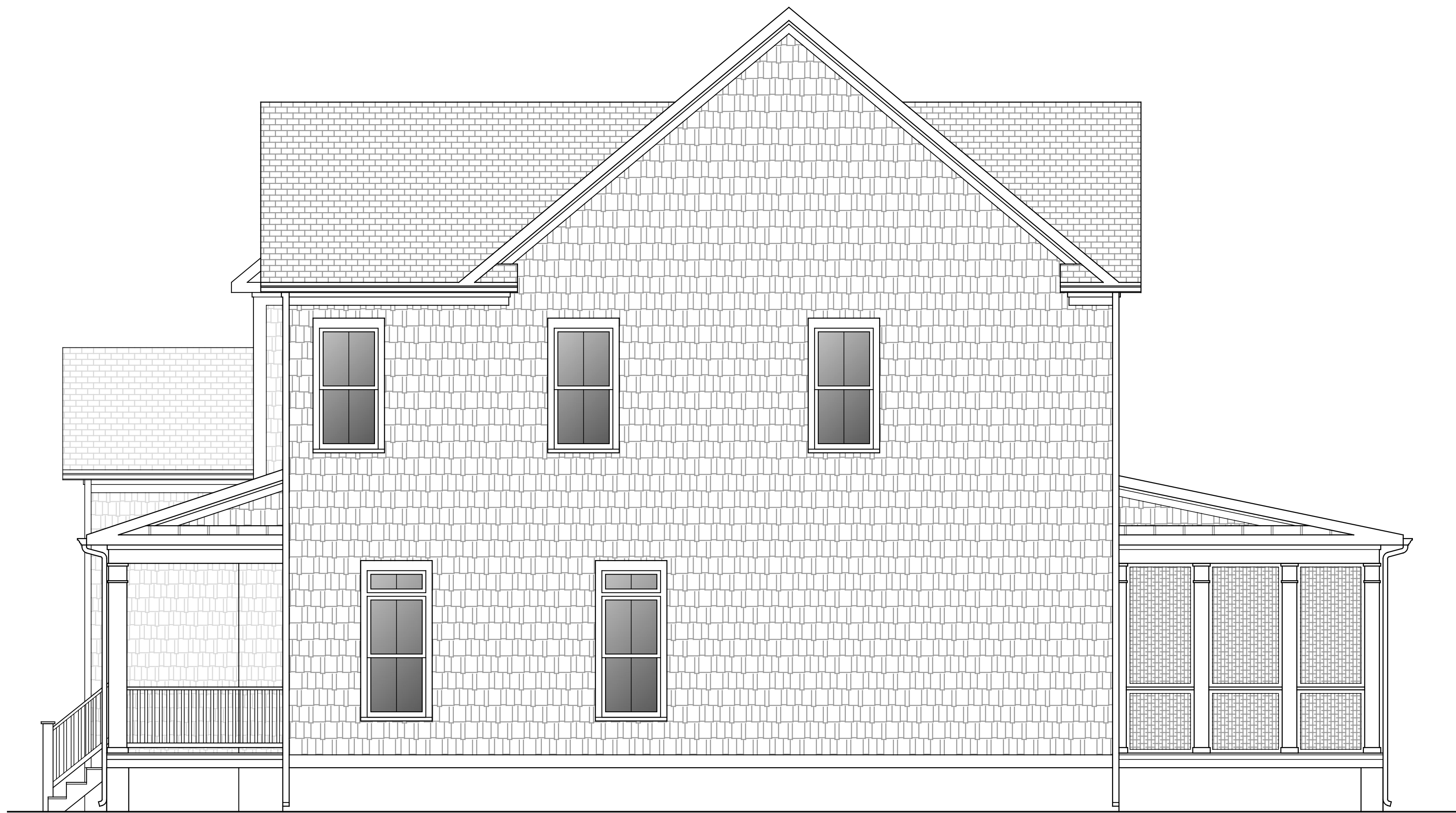
01 | RIGHT SIDE ELEVATION 1/4" = 1'
