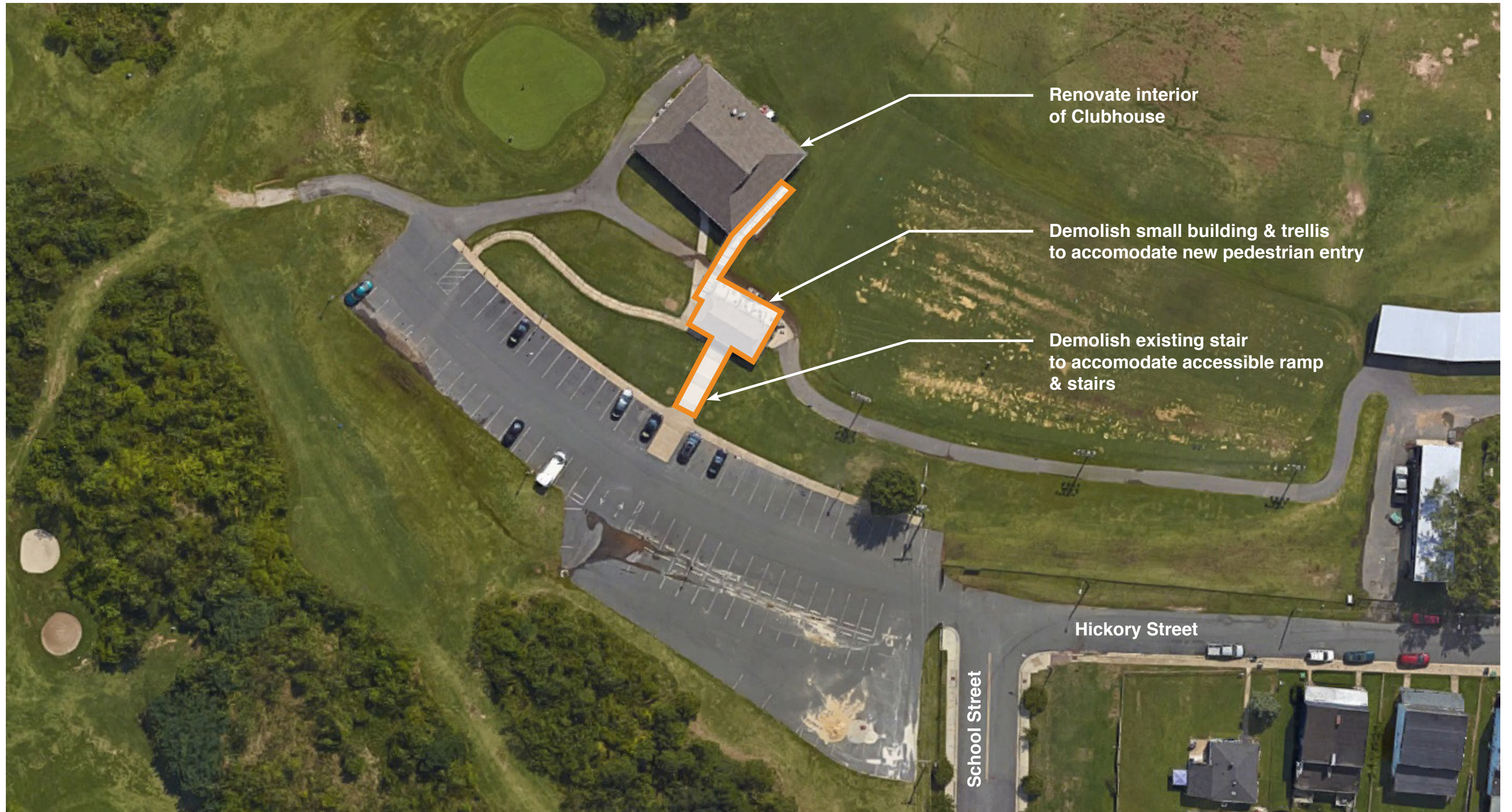
existing site plan with proposed demolition
