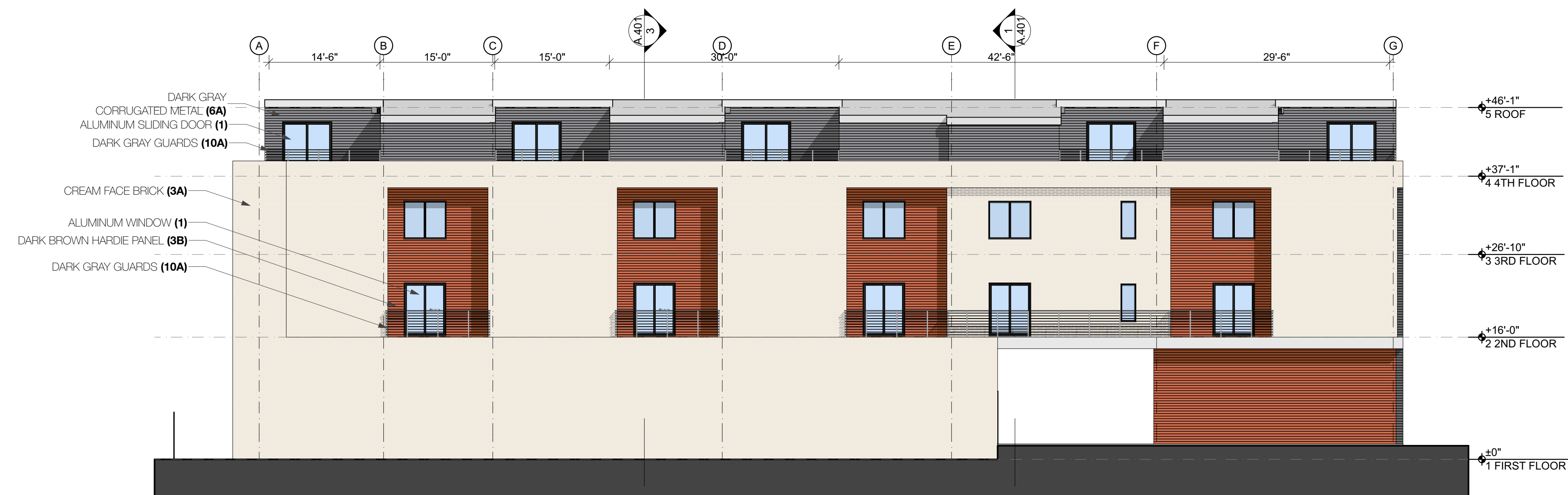
2 NW COLOR ELEVATION SCALE: 3/32" = 1'-0"
