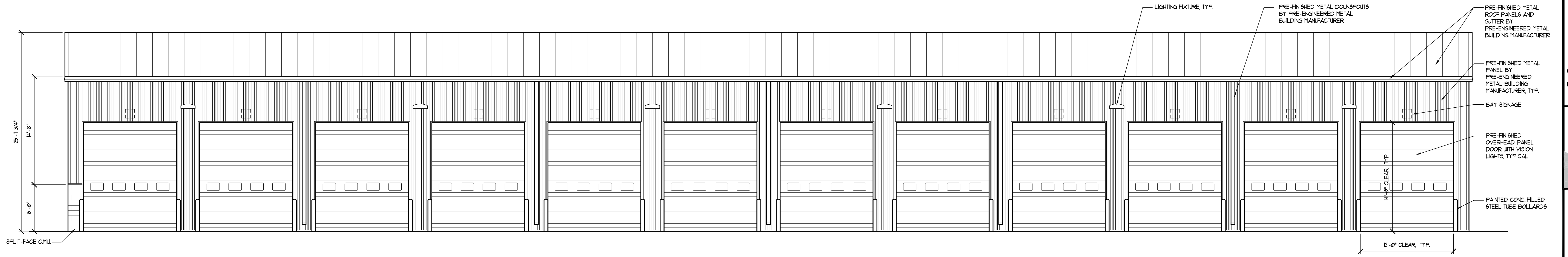
4 BUILDING 2 - SOUTH ELEVATION SCALE: 3/16" = 1'-0"
