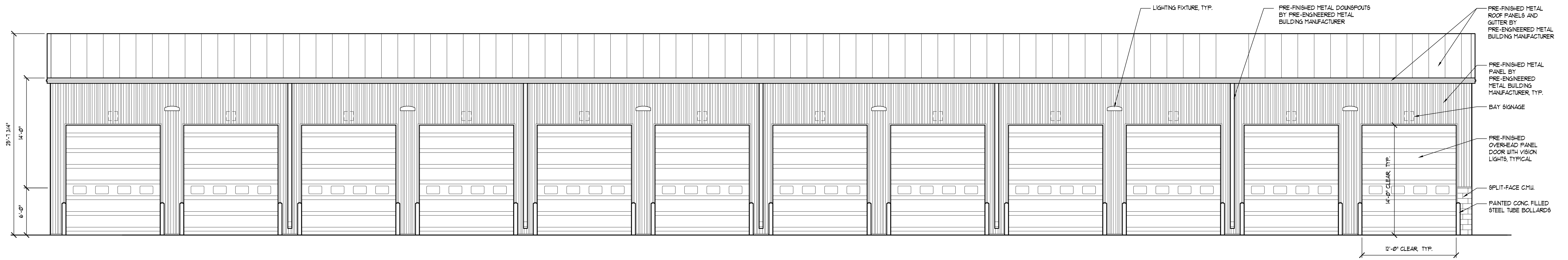
3 BUILDING 2 - NORTH ELEVATION SCALE: 3/16" = 1'-0"
