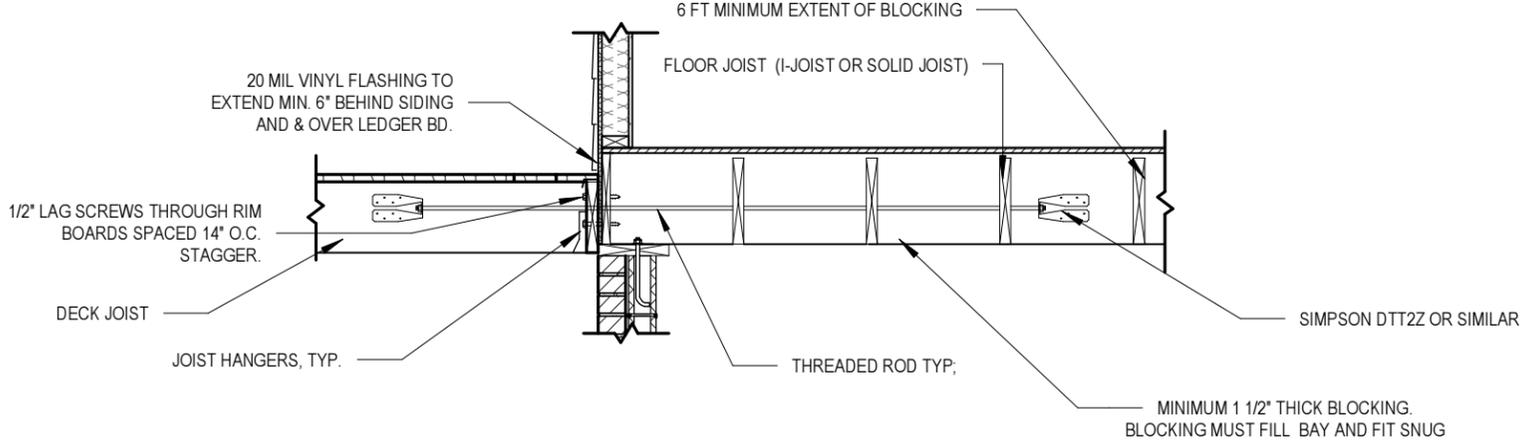
**3 DECK ATTACHMENT DETAIL DTT2Z STANDARD WITH PERPENDICULAR JOIST**
