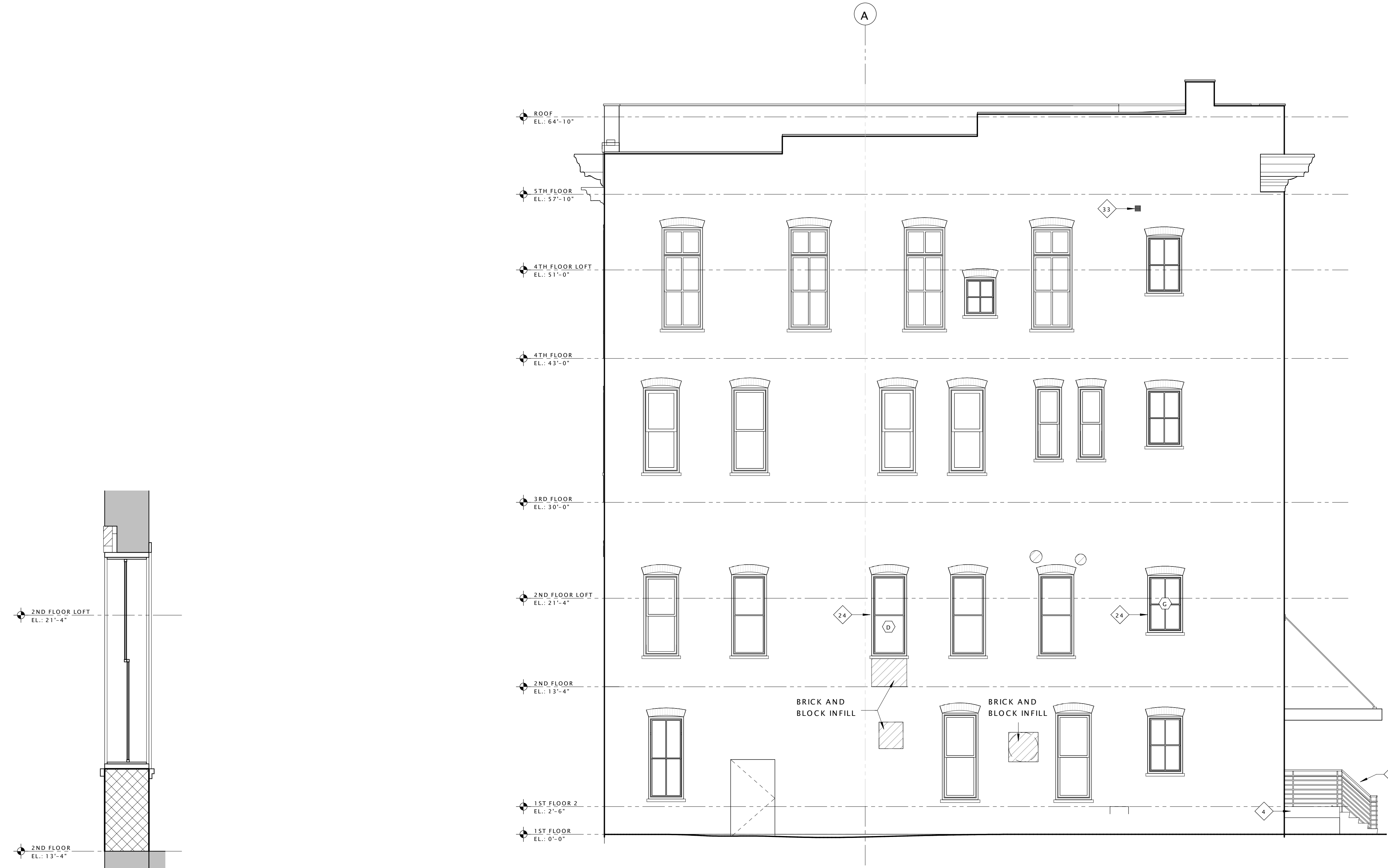
2 WEST ELEVATION - WALL INFILL DETAIL SCALE: 1/2" = 1'-0"
