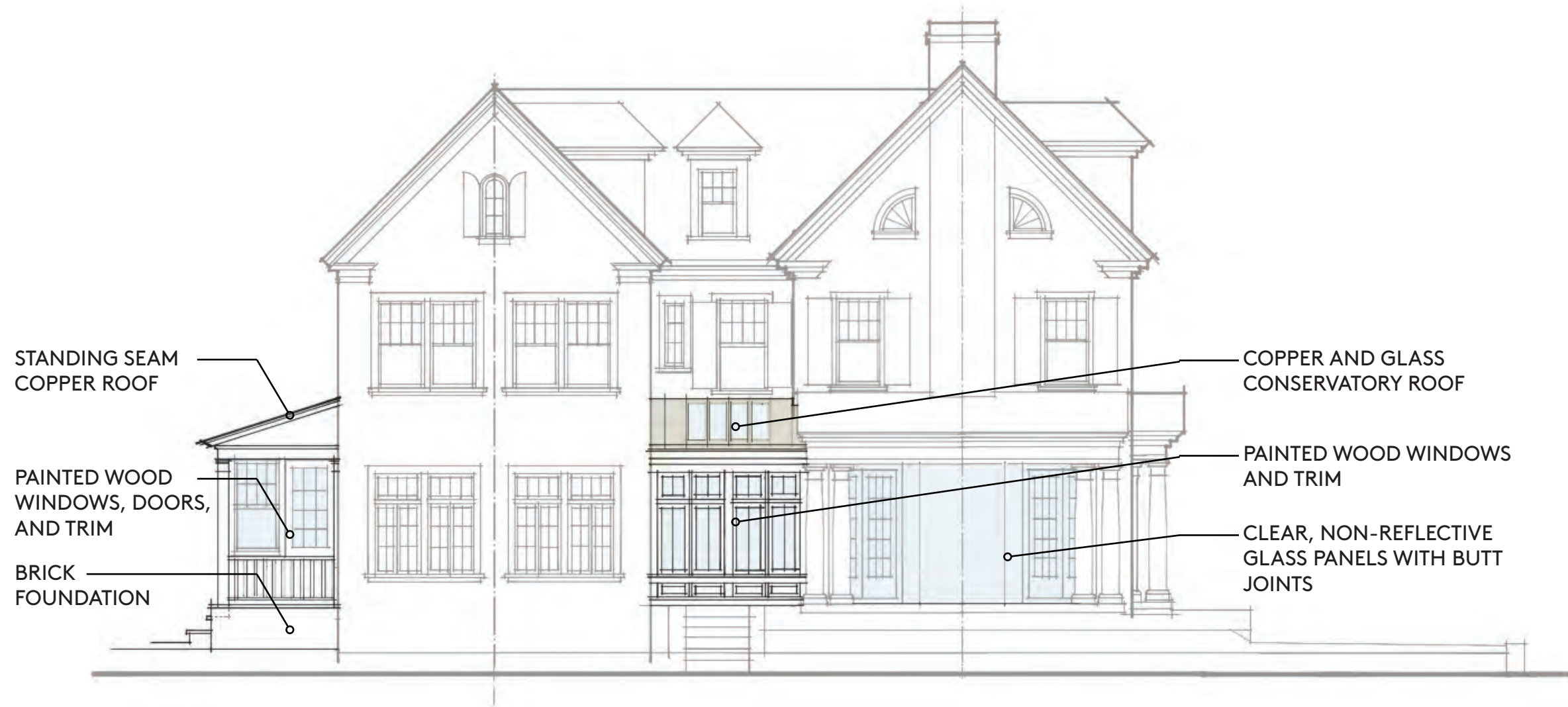
SOUTH ELEVATION (SECONDARY)
