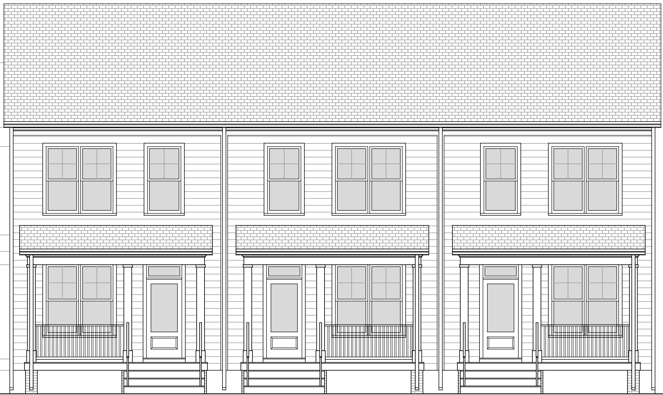
01 | FRONT ELEVATION - BUILDING A 1/4" = 1'
