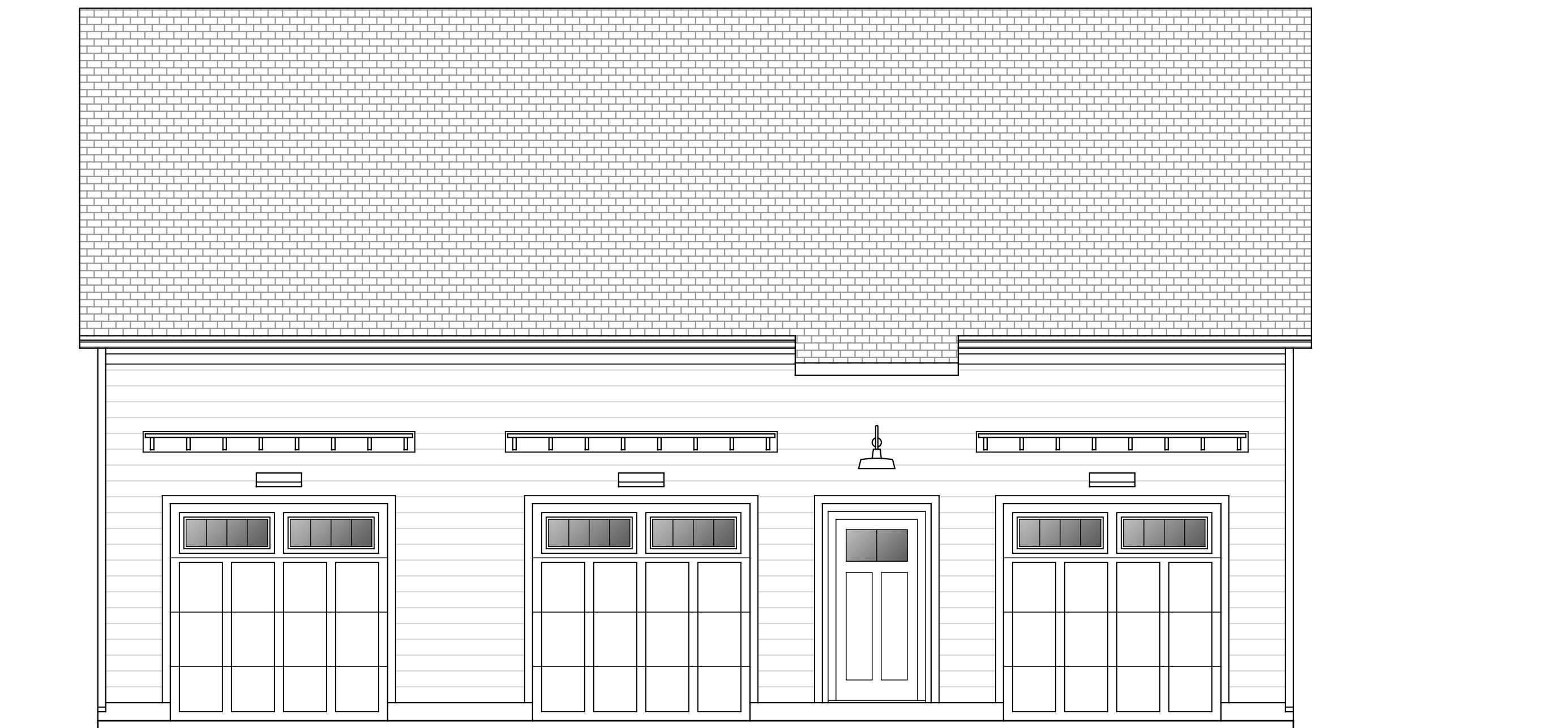
02 | GARAGE LEFT SIDE (ALLEY) ELEVATION 1/4" = 1'
