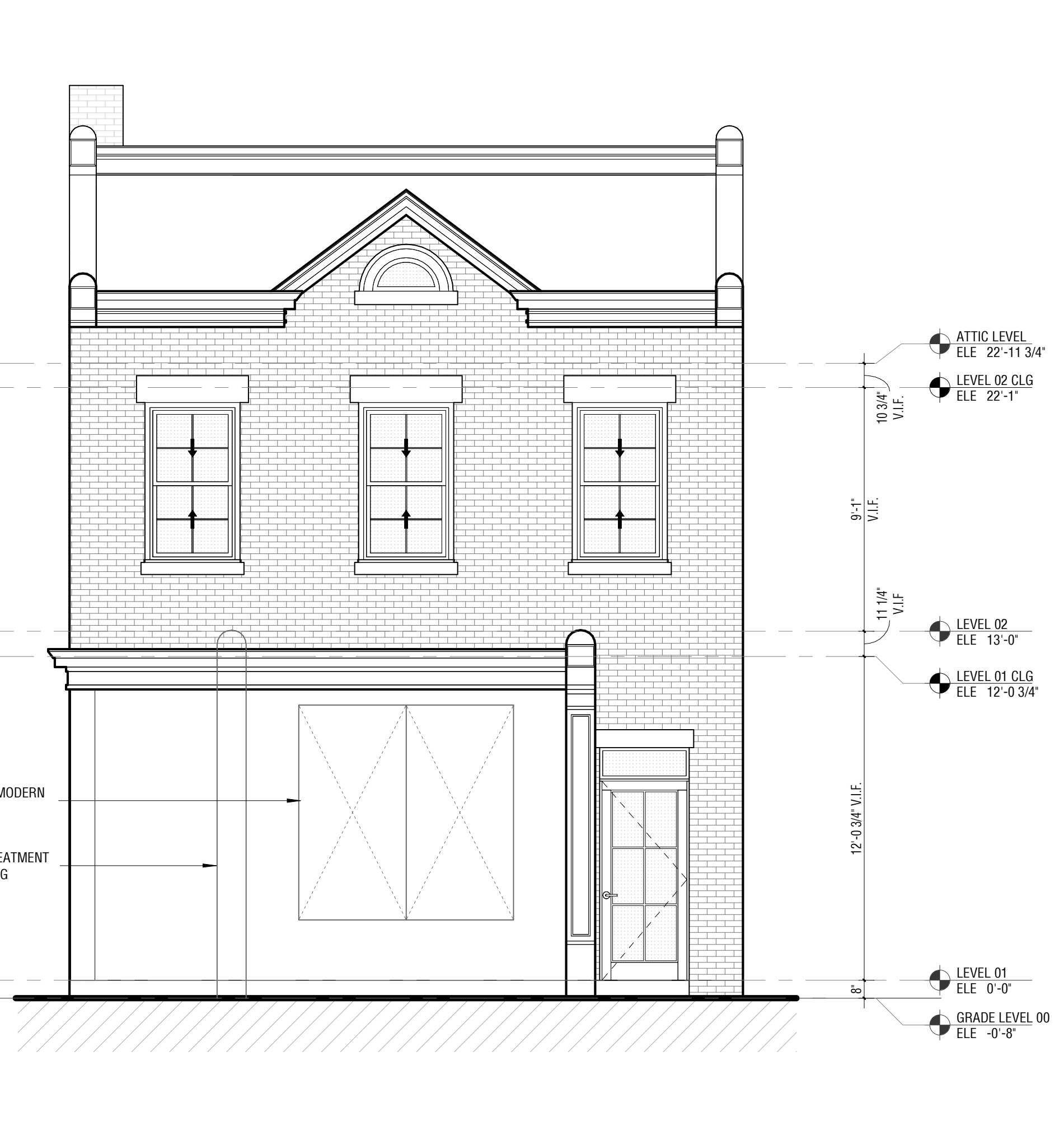
01 EAST BUILDING ELEVATION SCALE: 1/4" = 1'-0"
