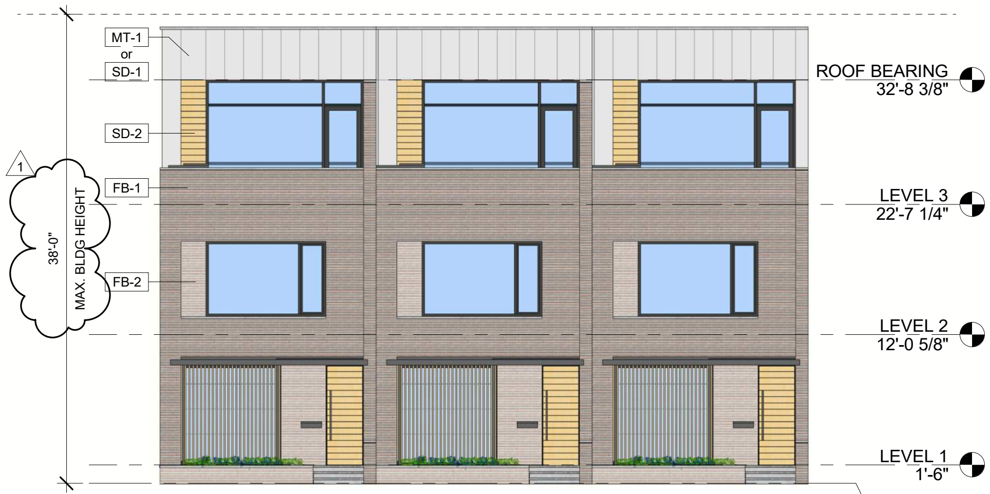
2 NORTH ELEVATION - ALLEY P1.2 1/8" = 1'-0"
