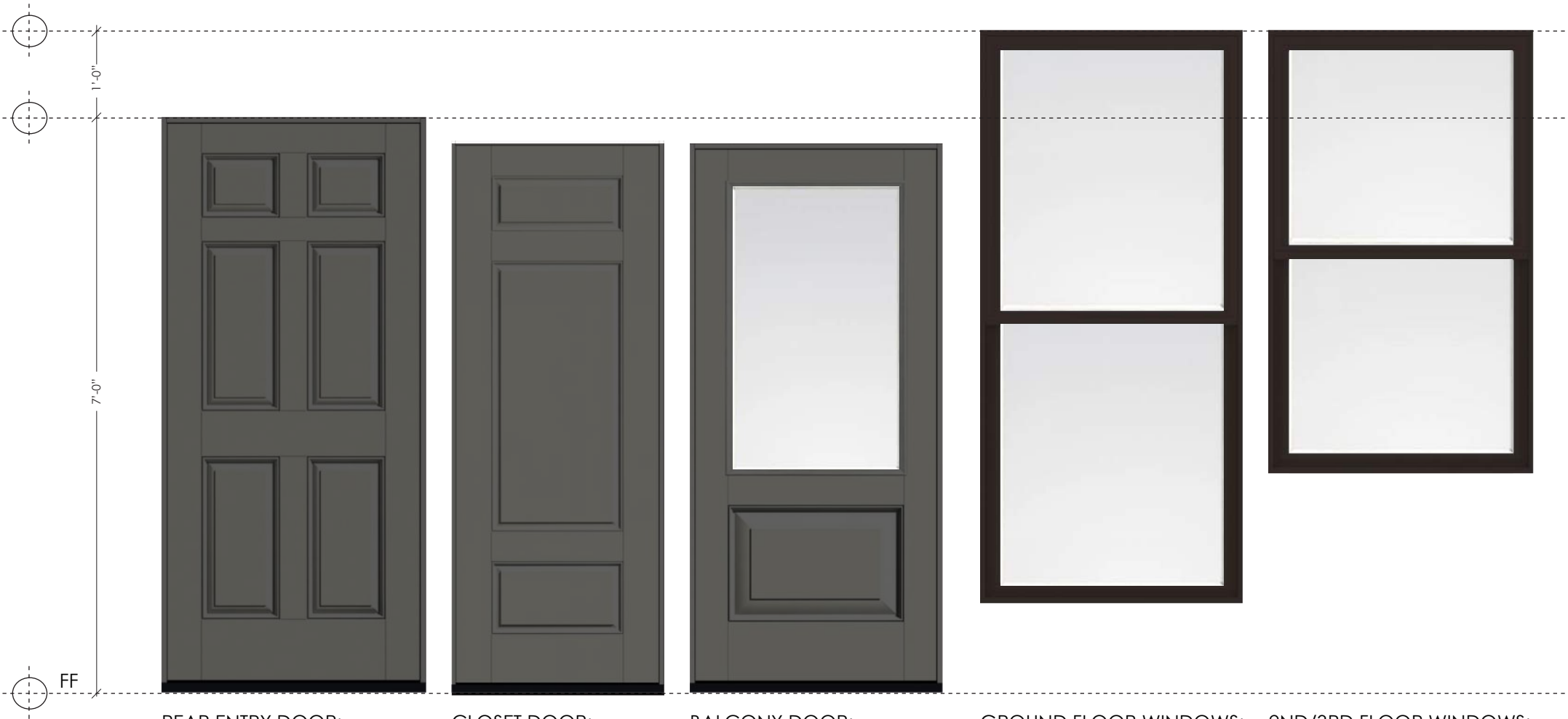
REAR ENTRY DOOR: THERMA-TRU FIBERGLASS CLASSIC CRAFT FOUNDERS COLLECTION 3-0 7-0
