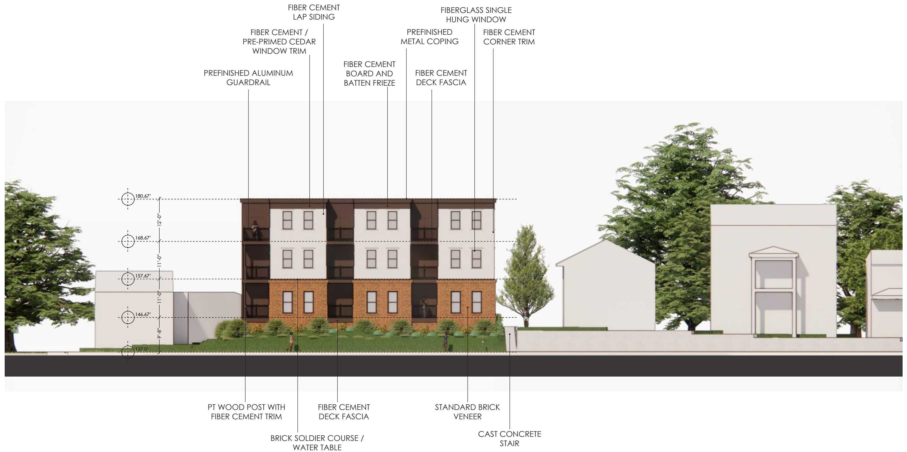
○ WEST ELEVATION SCALE: 3/32" = 1'-0"
