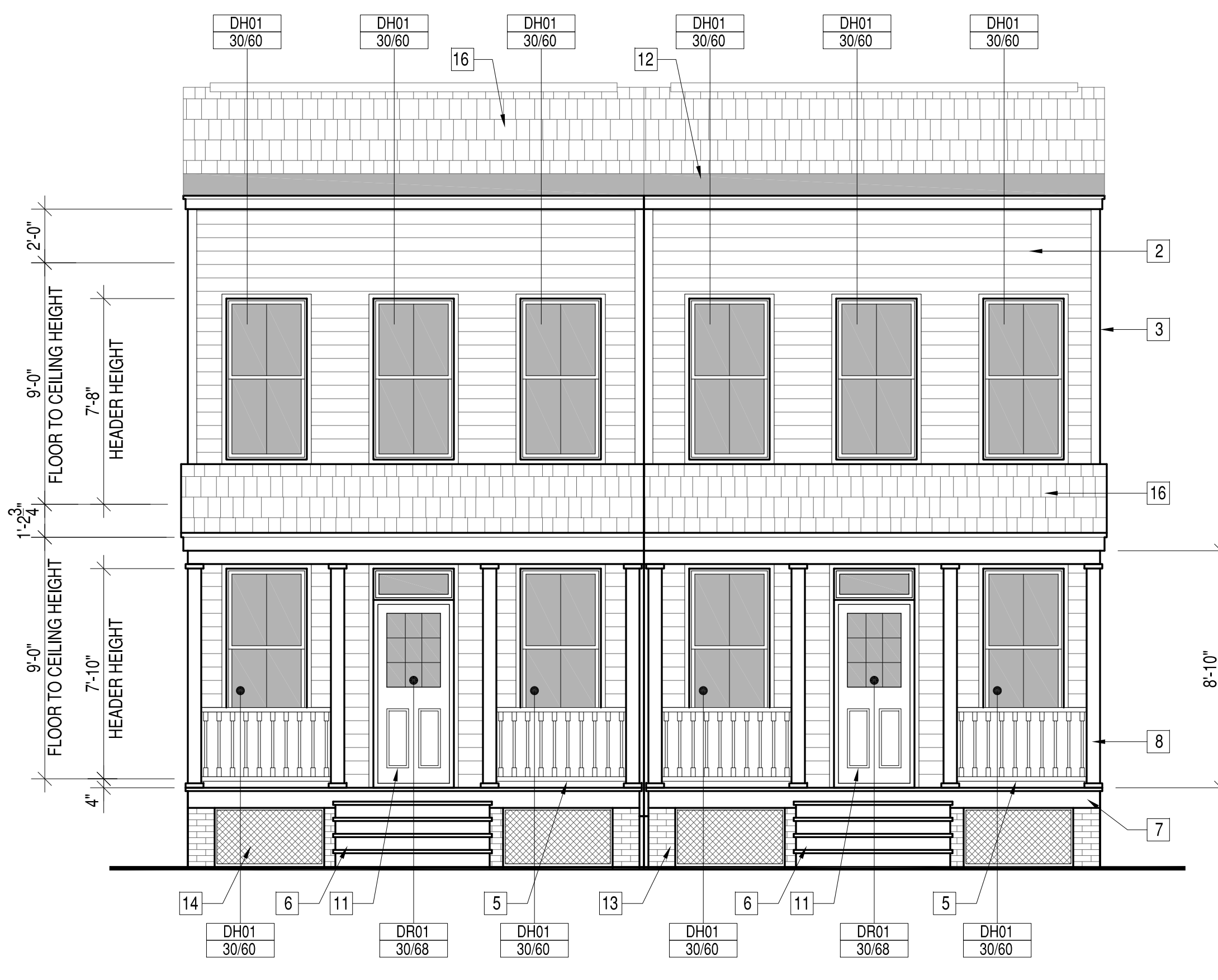
REAR ELEVATION - SECTIONS 1 AND 4
