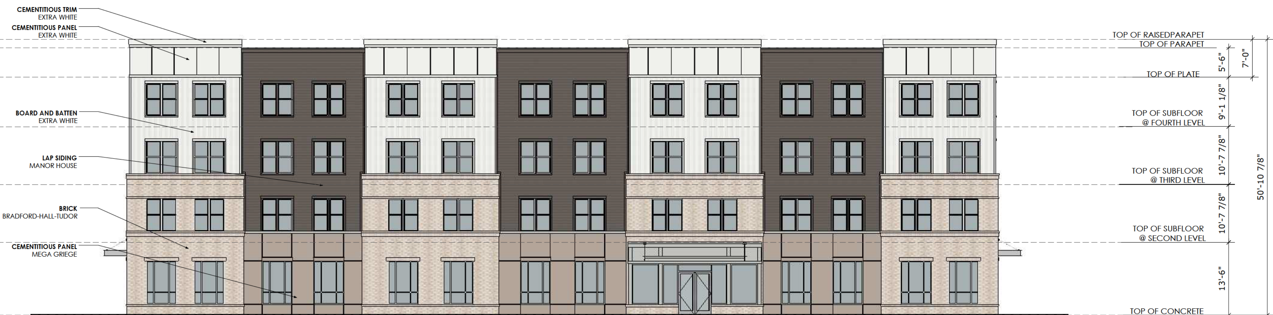
1 Multifamily - Building Type 1 - Front Elevation Scale: 3/32" = 1'-0"
