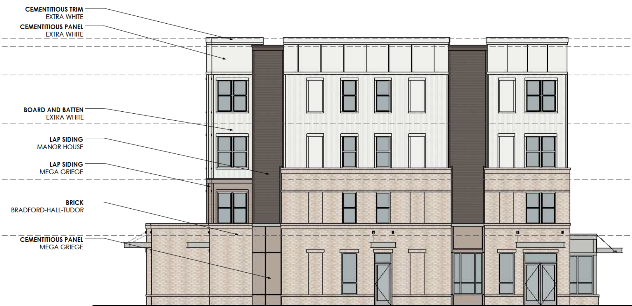
2 Multifamily - Building Type 1 - Left Elevation Scale: 3/32" = 1'-0"
