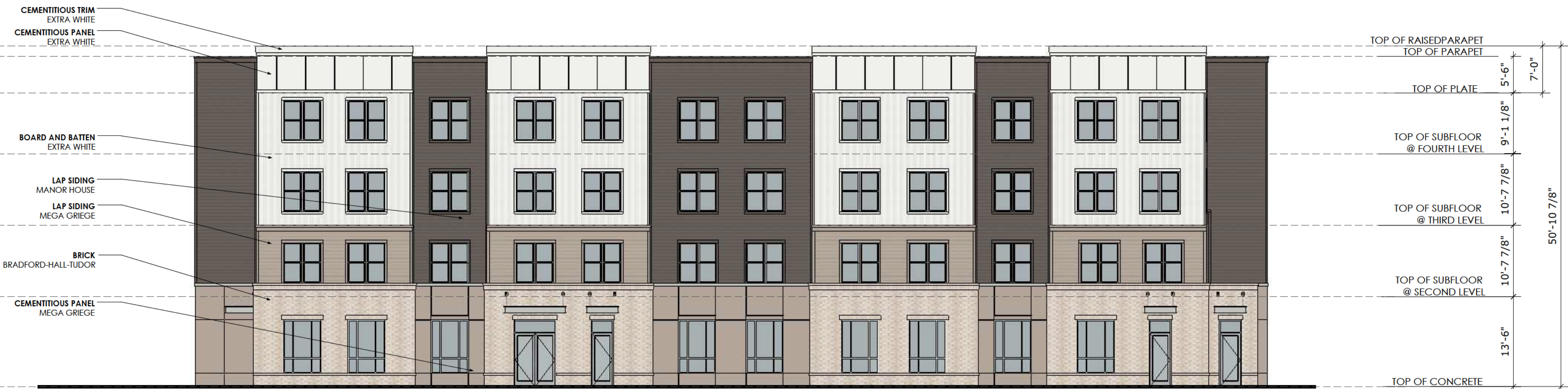
3 Multifamily - Building Type 1 - Back Elevation Scale: 3/32" = 1'-0"
