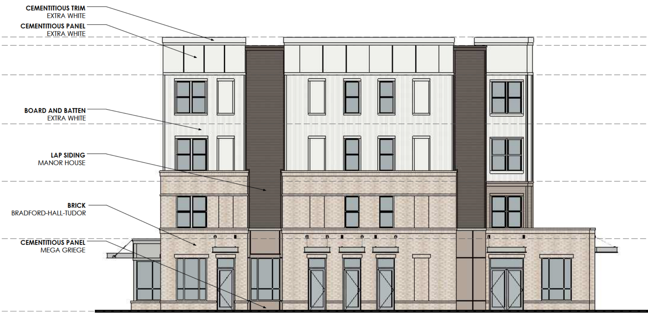
4 Multifamily - Building Type 1 - Right Elevation Scale: 3/32" = 1'-0"
