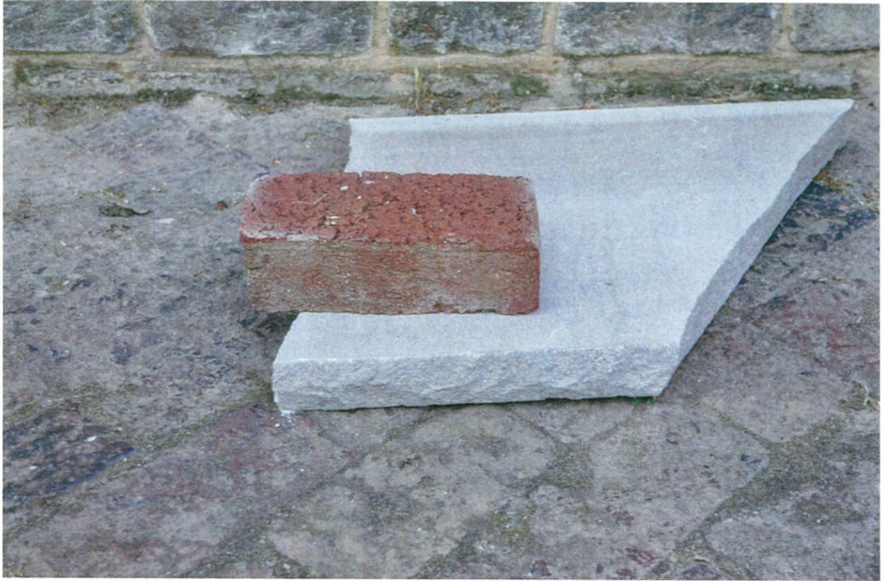
brick sample for garden walls and limestone cap
