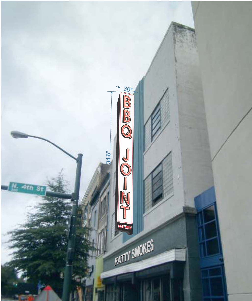
Channel letters red neon sign. Clear plexiglass faces, red neon lighting, black trim caps, black returns. Sizes and colors as depicted on the drawing.
