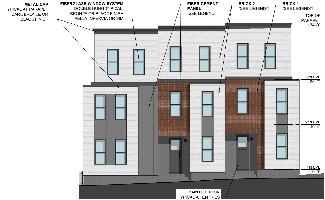
GROUPING 02 | SOUTH ELEVATION (FACING E BROAD ST) 2s
