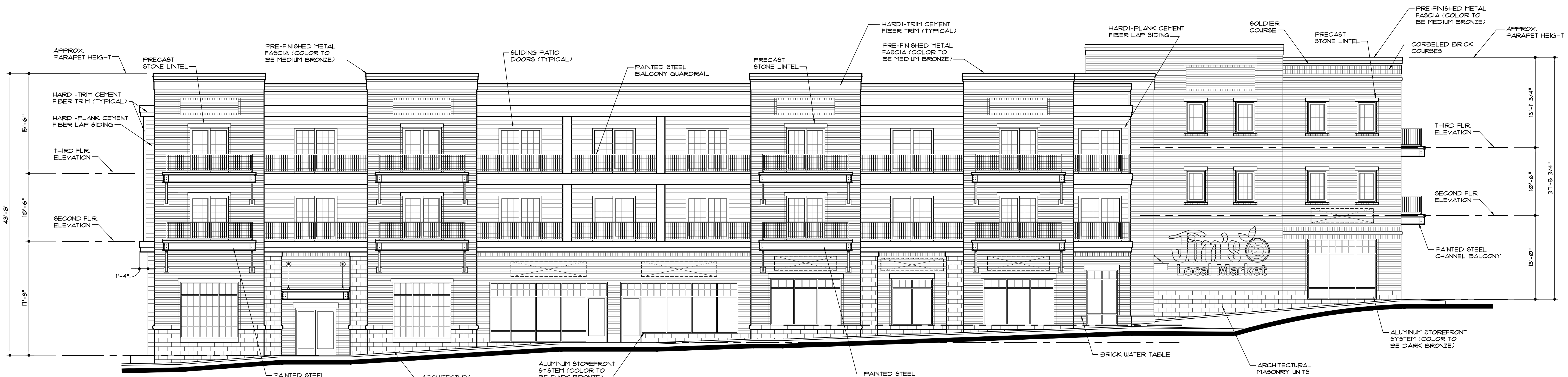
SOUTHWEST ELEVATION (FAIRMOUNT AVE.) SCALE: 1/8" = 1'-0"
