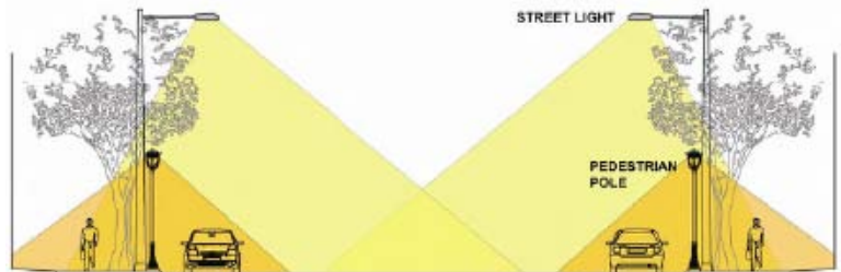
Figure 6 Street and Pedestrian Lighting
