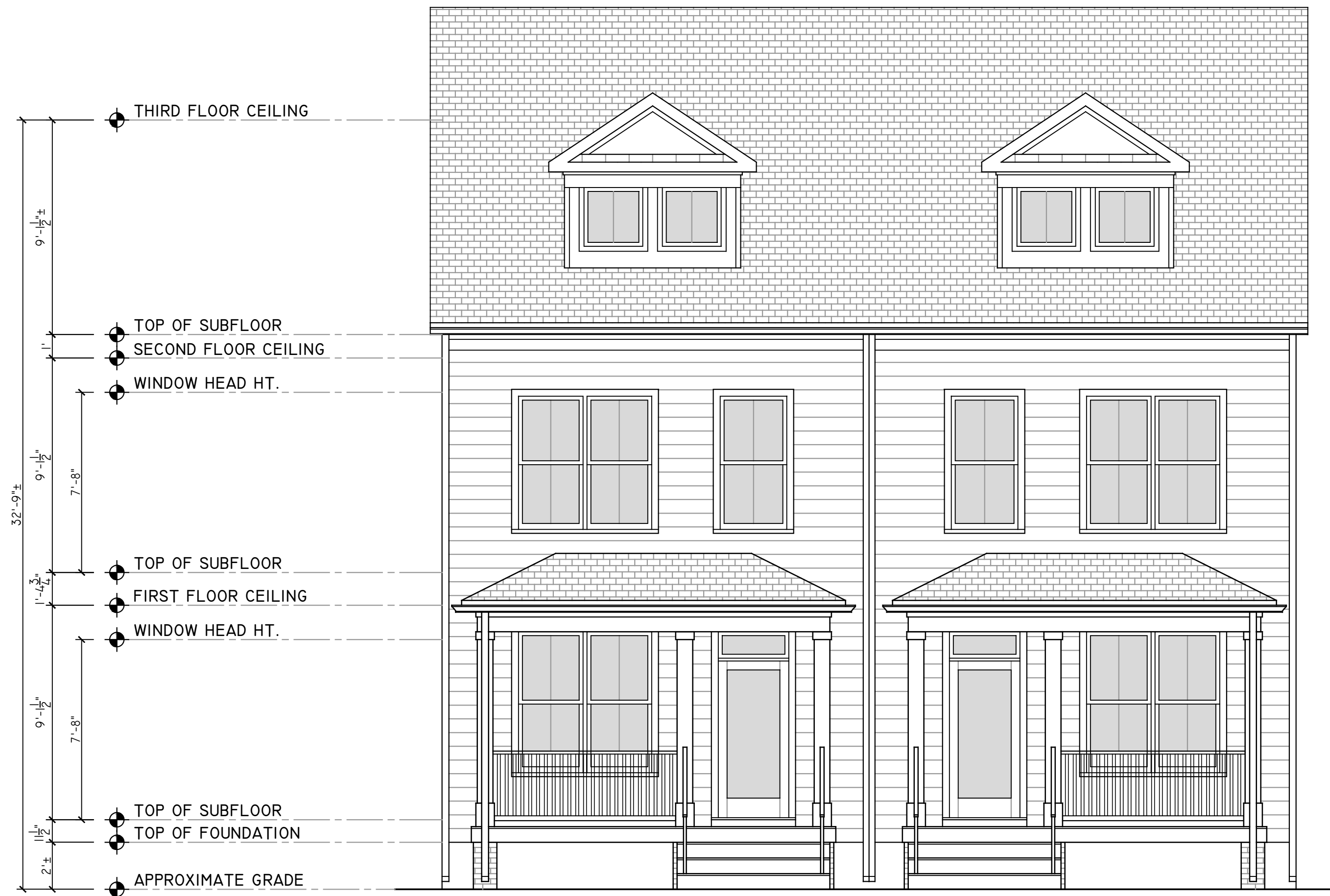
02 | FRONT ELEVATION - BUILDING B 1/4" = 1'
