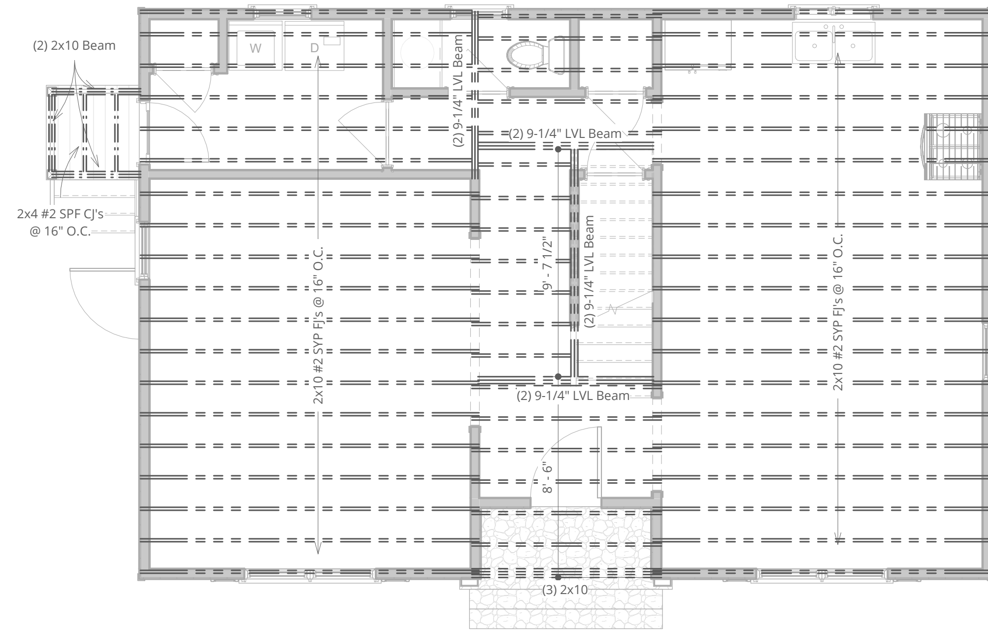
1st FLOOR CJ FRAMING PLAN 1/4" = 1'-0"
