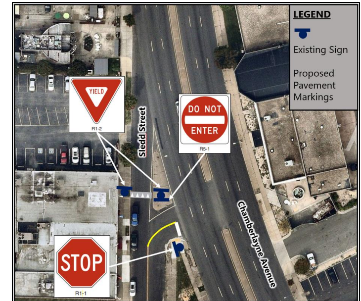
Sledd Street intersection signing and marking recommendations
