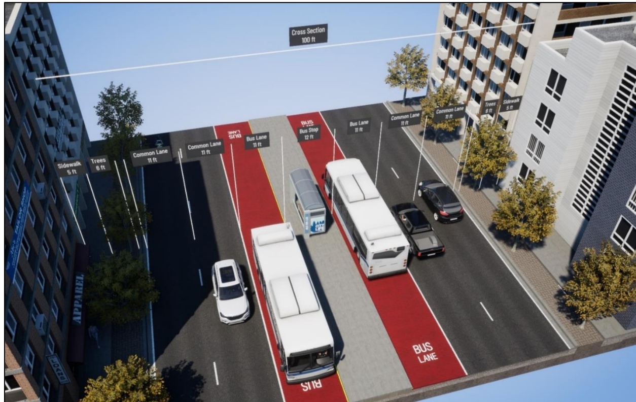
Potential Bus Rapid Transit 100-foot Cross-Section
