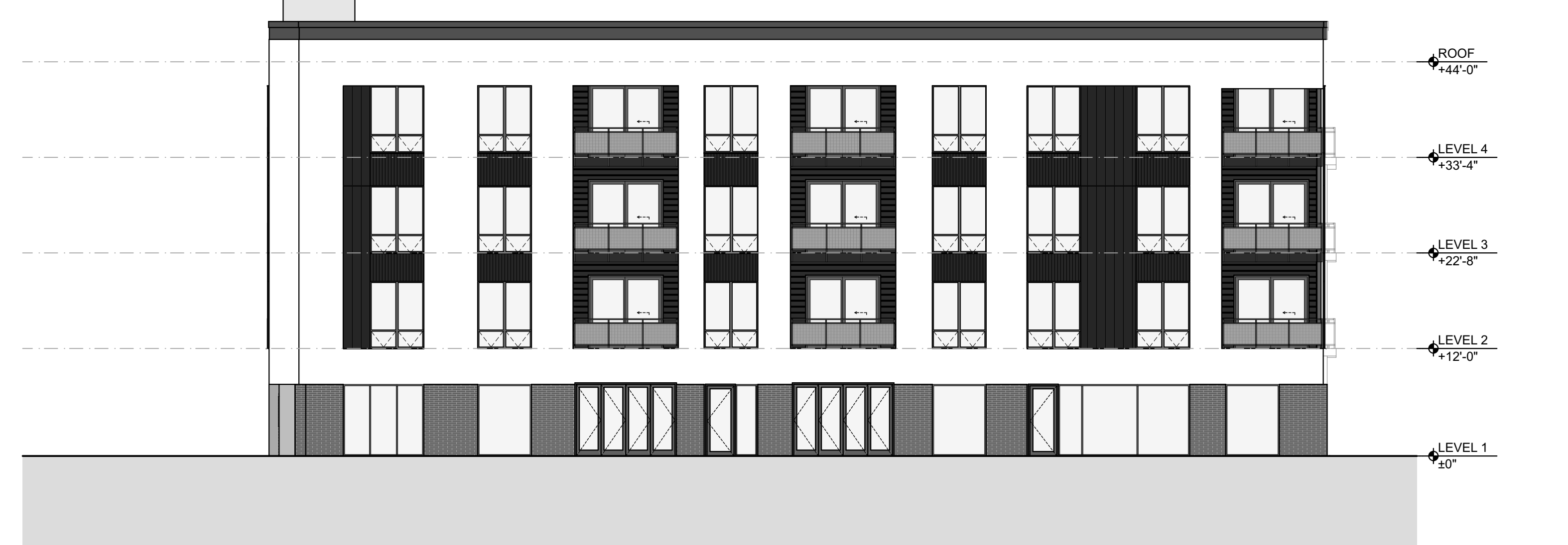
BUILDING A EAST ELEVATION 3 SCALE: 3/32" = 1'-0" A200
