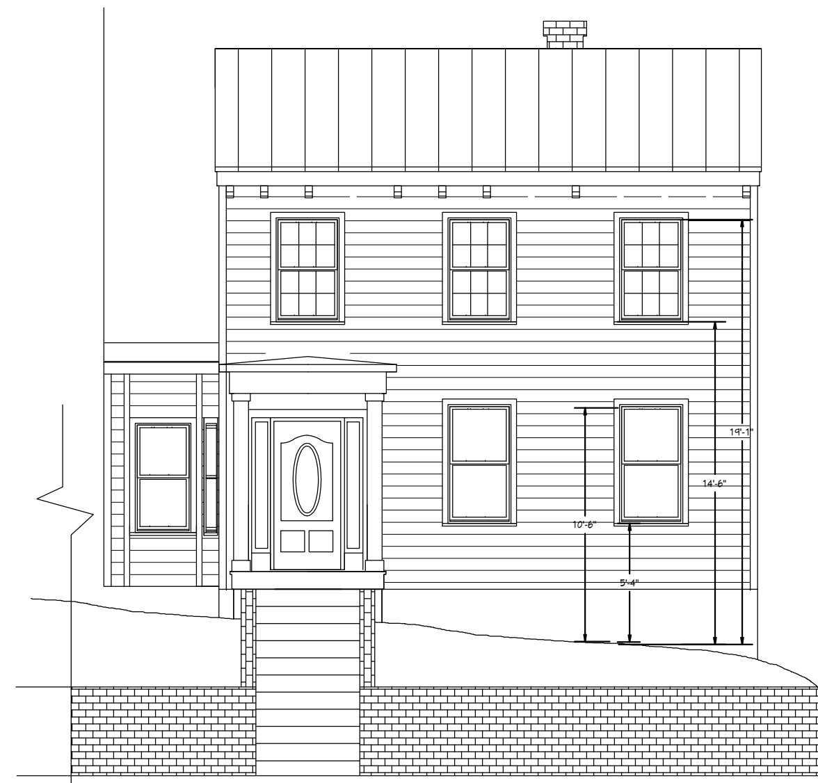
1 FRONT ELEVATION: EXISTING CONDITIONS 2 CEDAR AVE PROJECT 3/16"=1'-0"
