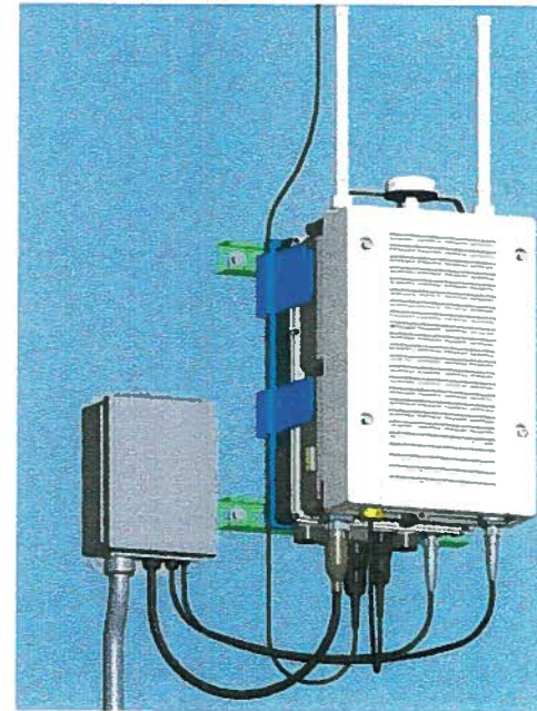
Antenna/equipment cabinet micro design
