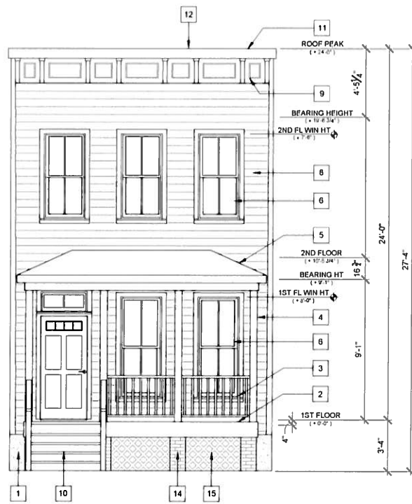
FRONT ELEVATION SCALE: 1/4"=1'-0"
