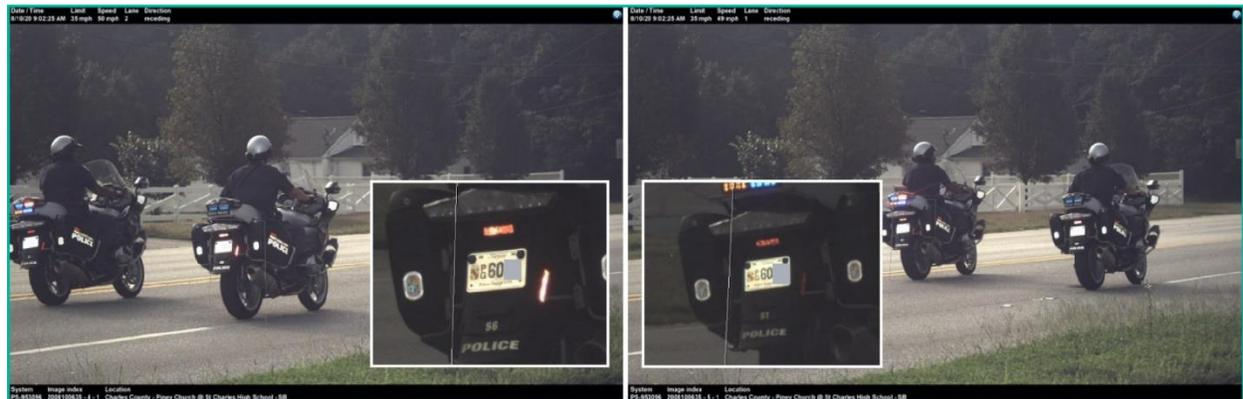
**Figure 4.16-3. Capturing Simultaneous Violations within the Same Lane**
