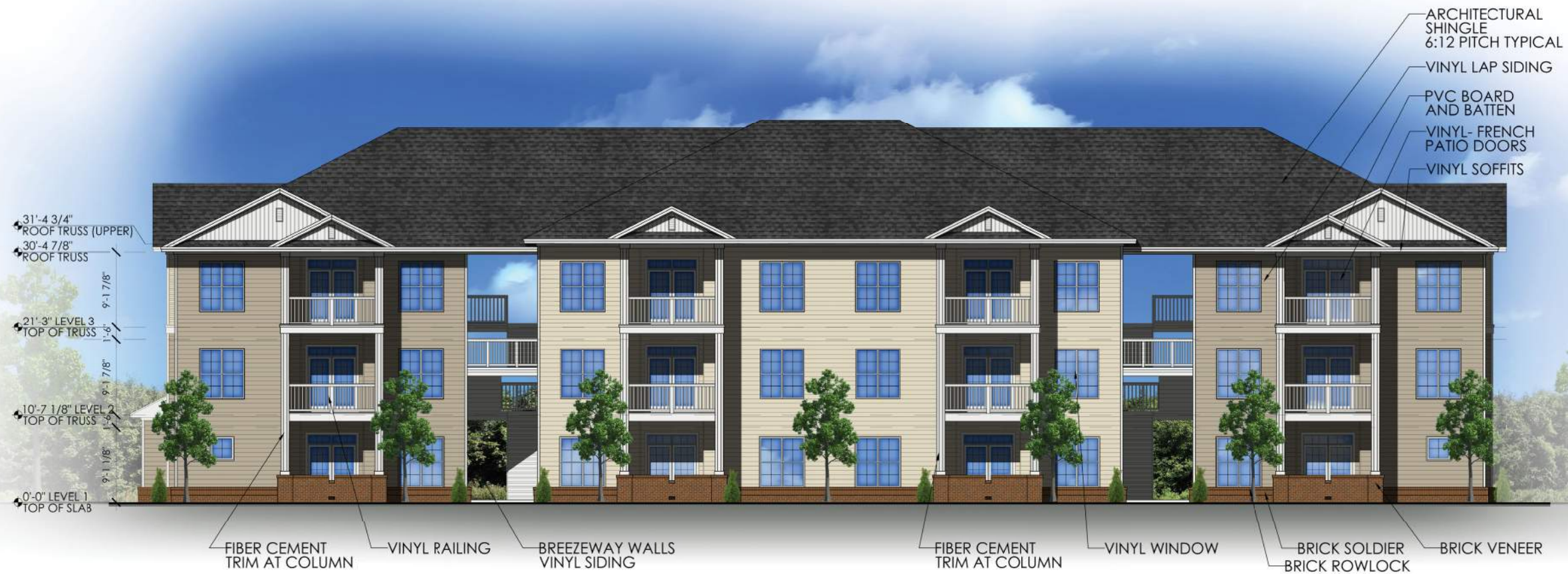
TYPE 1 - REAR BUILDING ELEVATION
