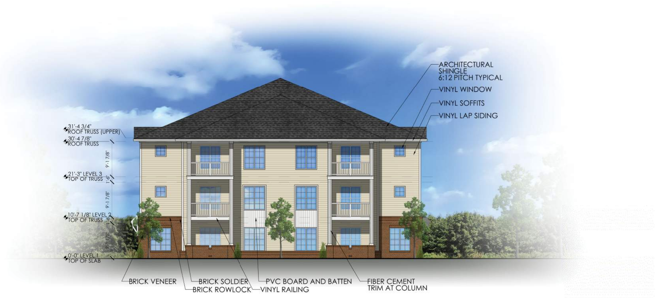
TYPE 4 - SIDE BUILDING ELEVATION
