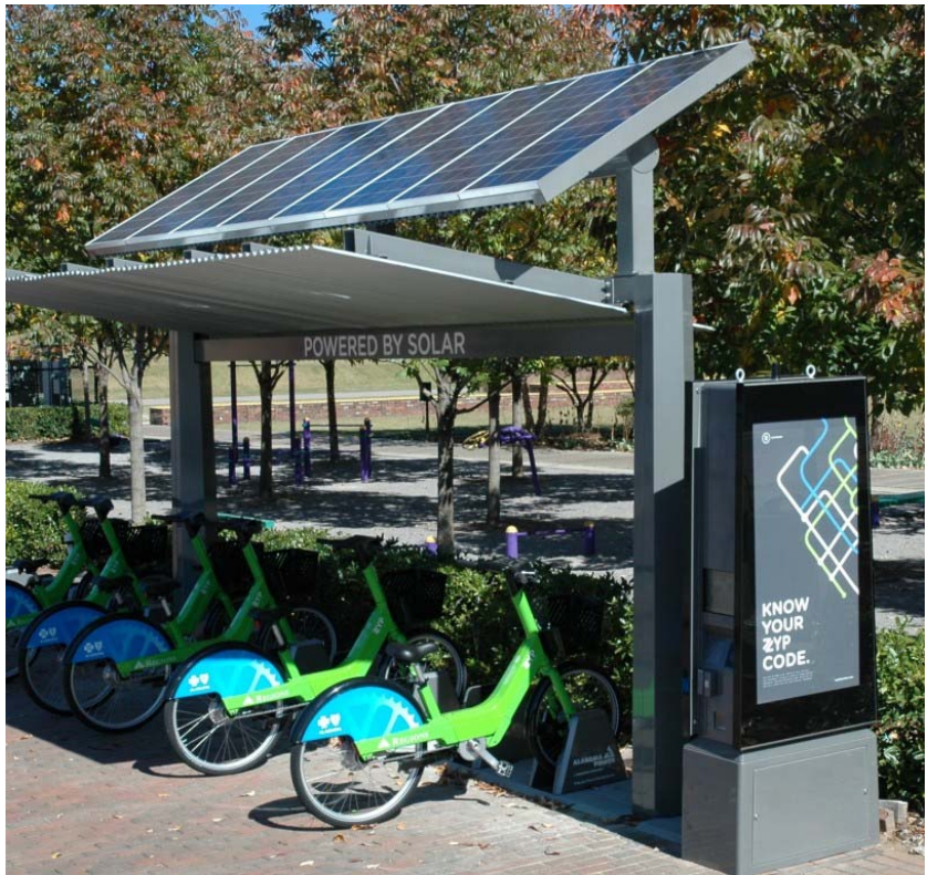
Solar charging canopy for pedelec (Phase II)
