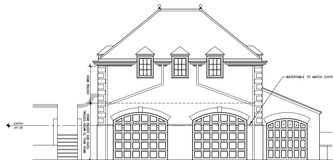
4 GARAGE PAVILION EAST ELEVATION SCALE: 1/4" = 1'-0"
