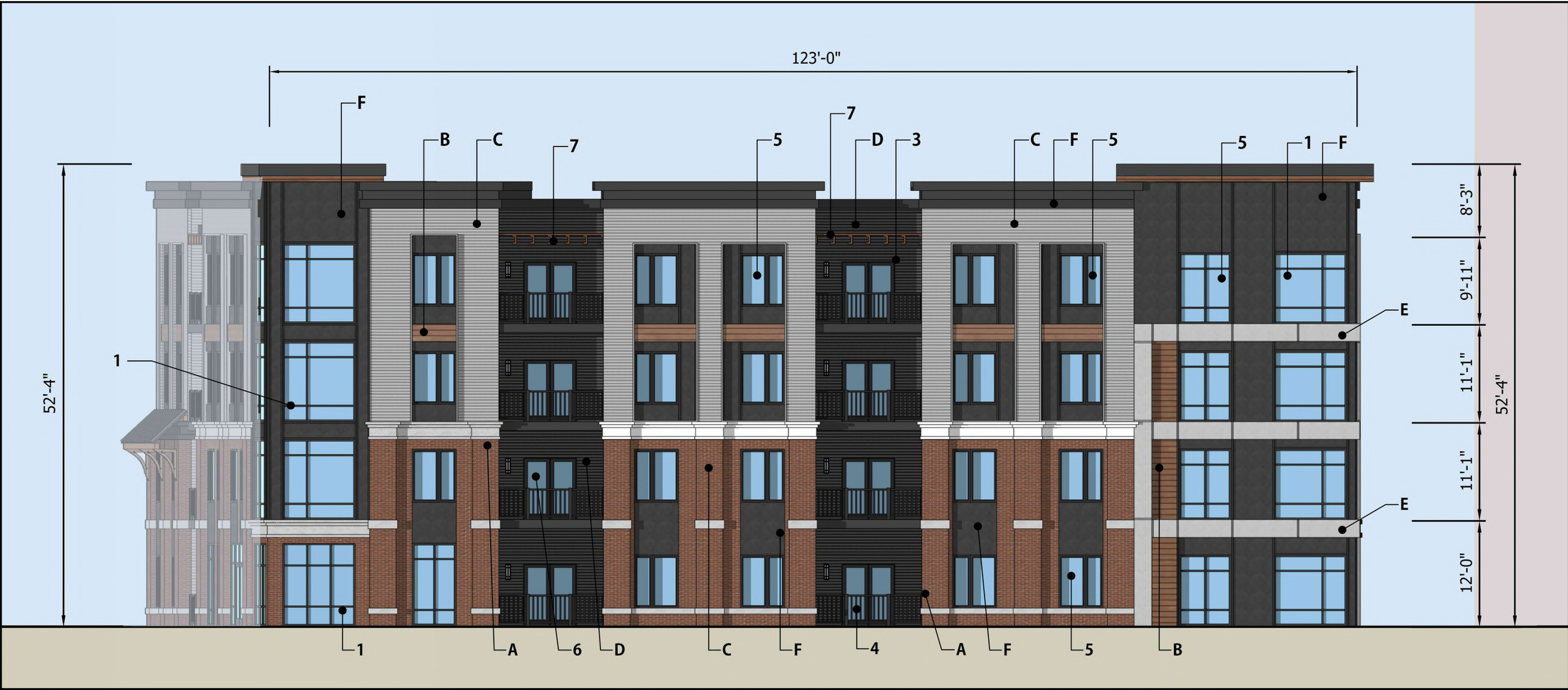
1 ENLARGED NORTH ELEVATION / MATERIALS (OVERBROOK RD) 3/16"=1'-0"
