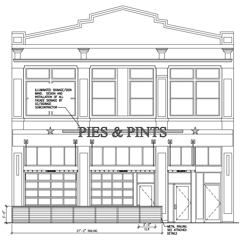
5 NORTH ELEVATION (STREET) - PROPOSED SIGNAGE & RAILING SCALE: 1/4" = 1'-0"
