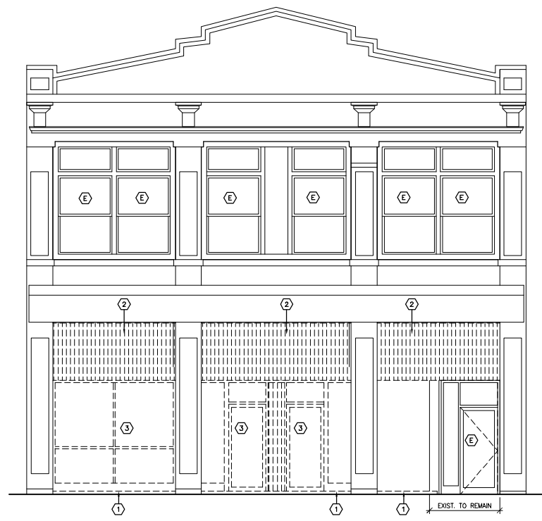
1 NORTH ELEVATION (STREET) - DEMOLITION SCALE: 1/4" = 1'-0"
